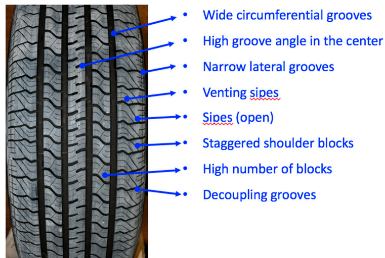
Figure 19. Example of a tread design with low TPIN characteristics (modified from Saemann, 2005 [159]; reprinted under fair use provision).
