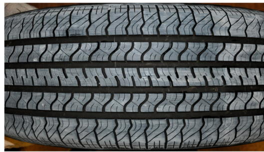
Figure 15. Tread pattern of SRTT (tread surface is white painted).
