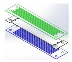
Figure 1. Exploded view of the three-layer bipolar plate.
