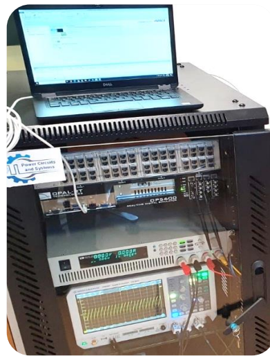
Figure 7. Photograph of the OPAL-RT setup adopted for the HiL verification.
