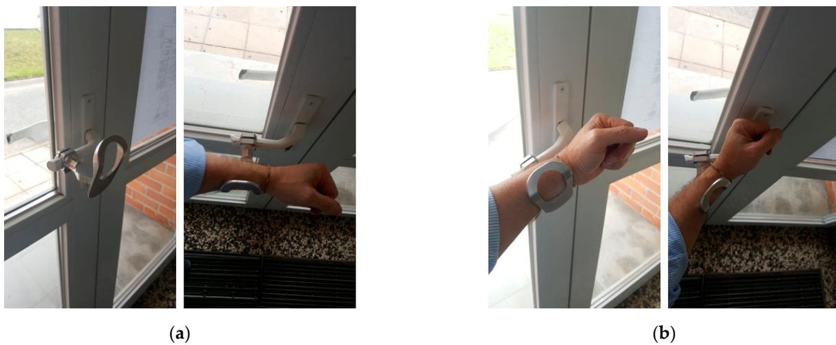
**Figure 16.** Dynamic system: (a) visualization of the system clamped in the handle and the hand position for opening; (b) sequence of opening performed by a volunteer.
