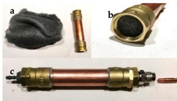
**Figure A4.** Flame-breaker assembly.
