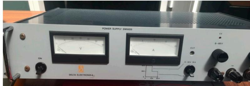
**Figure 4.** DELTA ELEKTRONIKA Power Supply SM6020 used for the dry cell tests.
