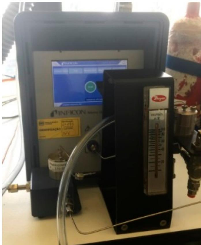
Figure 6. INFICON Micro GC Fusion.
