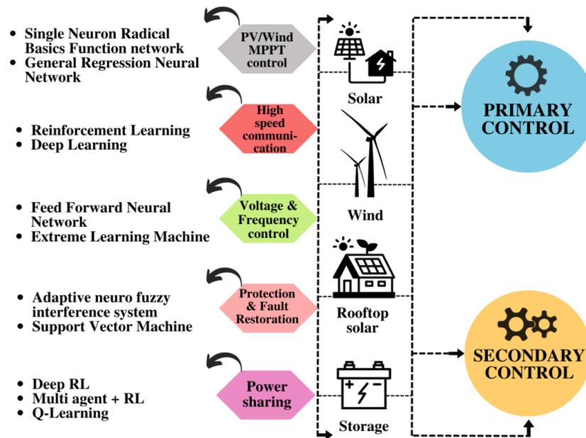
Figure 12. An outline of AI techniques in primary and secondary control and functionality of microgrids.
