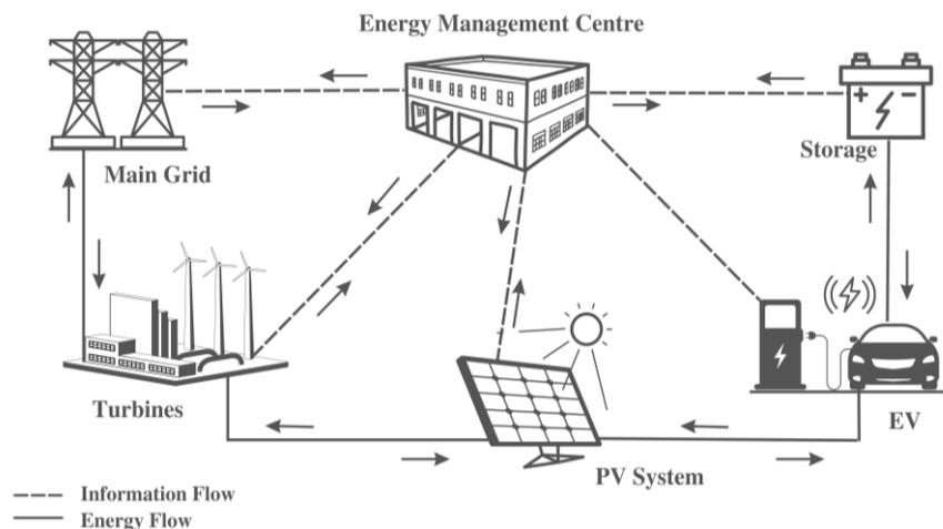
**Figure 1.** A typical schematic of a microgrid system.
