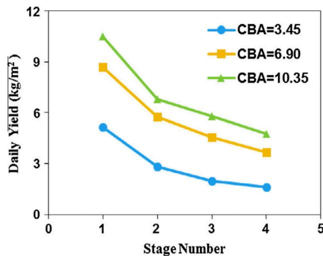
Figure 21. Differences in the daily distillation creation per unit area of the basin by different stages in the units with CBAs of 3.45, 6.90, and 10.35 [59] (License Number: 5373800957472).
