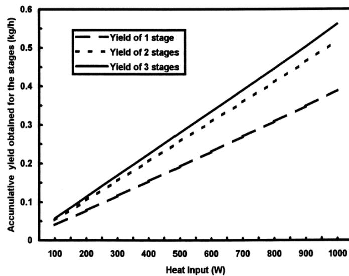
Figure 13. Accumulative yield of stages versus heat input [50] (License Number: 5373790205227).
