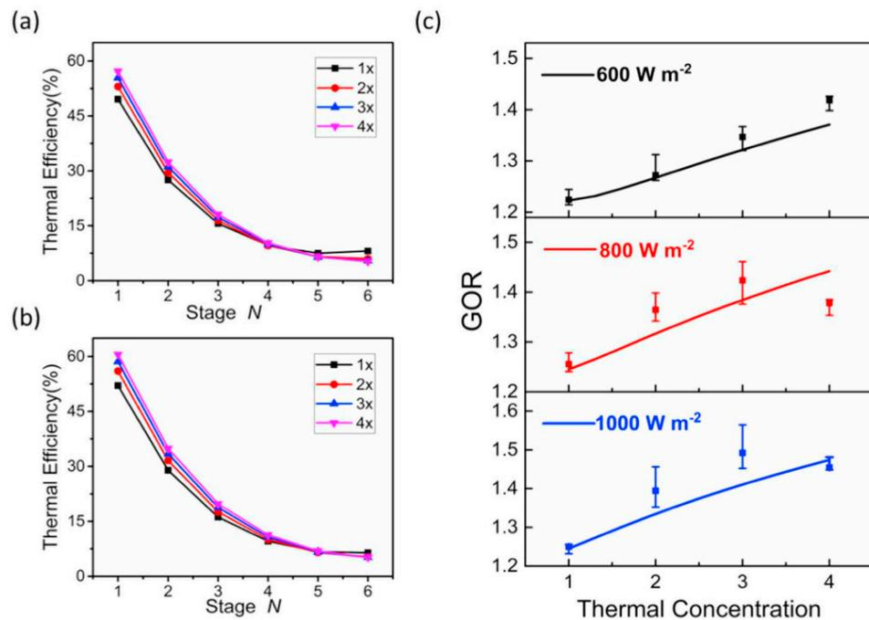
**Figure 18.** Designed thermal productivity of each stage under various radiation intensities: (a) 600 W m<sup>-2</sup> and (b) 1000 W m<sup>-2</sup>; (c) the GOR under various radiation intensities and heat loading, the dots correspond to the measured data, and the lines are the findings from theoretical model [56] (License Number: 5373840497196).
