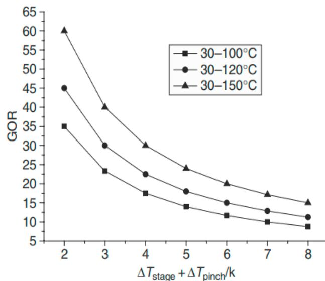
**Figure 5.** The GOR via the sum of the highest stages temperature variation and pinch point temperature change [41] (License Number: 5373820787675).
