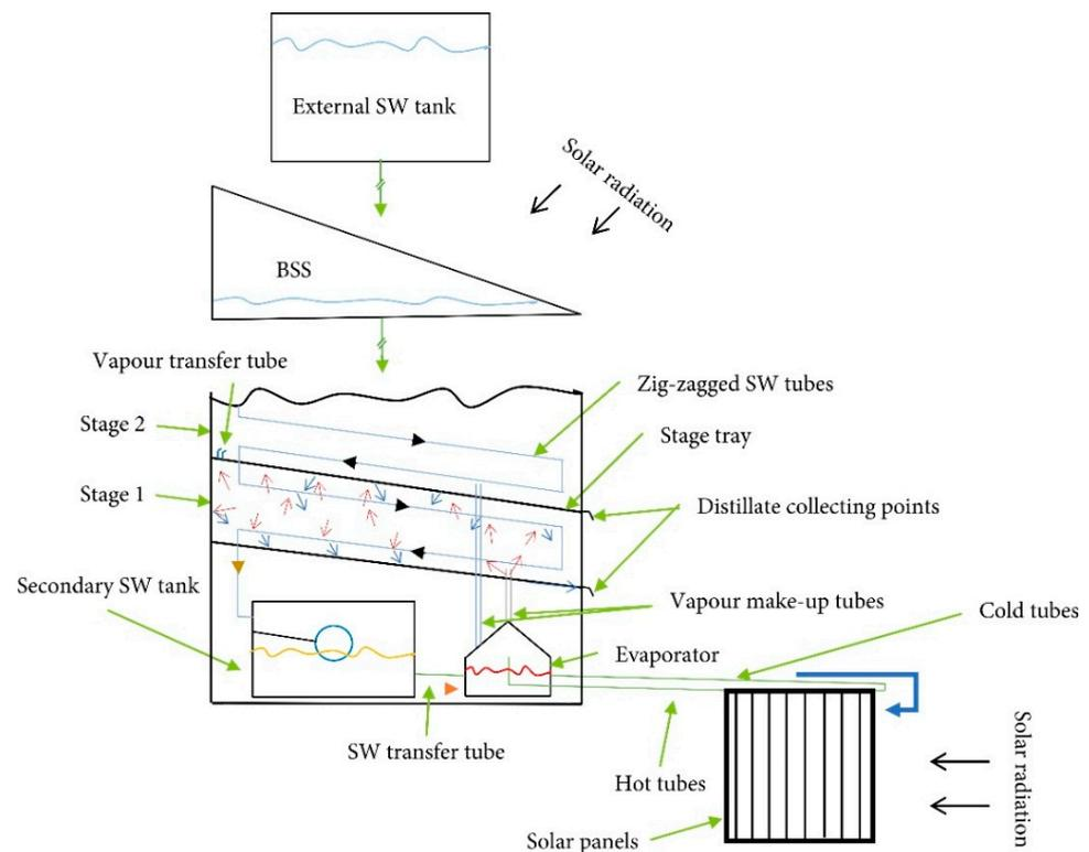
**Figure 2.** A schematic diagram of packed-tray multistage solar stills [35].
