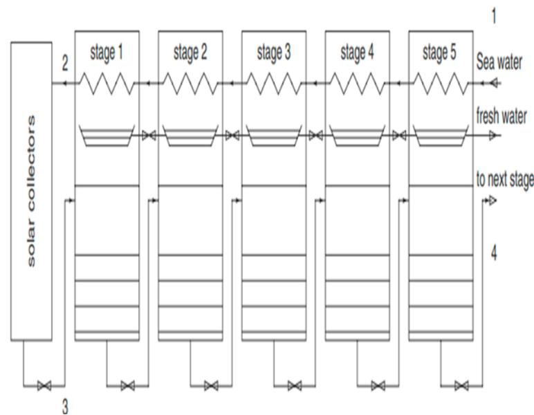
**Figure 4.** Diagram of the first five stages of the solar MSF distillation method [41] (License Number: 5373820787675).
