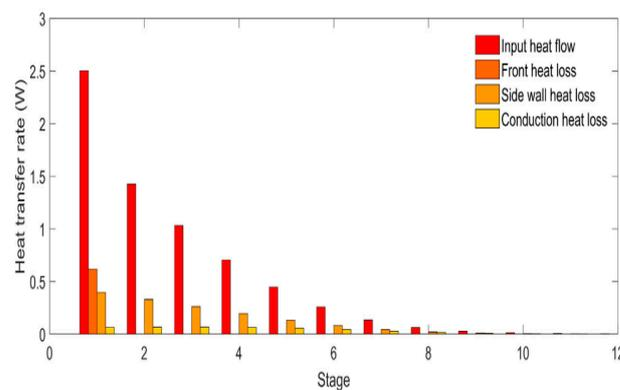
**Figure 17.** Heat transfer rate and different thermal losses at every system stage [55] (License Number: 5373820139387).
