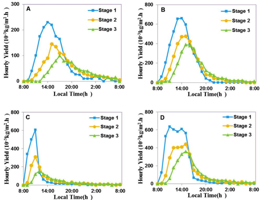
**Figure 22.** The rate of the clean water production when (A) 13 MJ energy was supplied, based on the regular solar irradiation design; (B) 27 MJ energy was consumed, based on the daily solar irradiation design; (C) 13 MJ energy was consumed spontaneously; (D) 27 MJ energy was consumed spontaneously [60] (License Number: 5373830138142).
