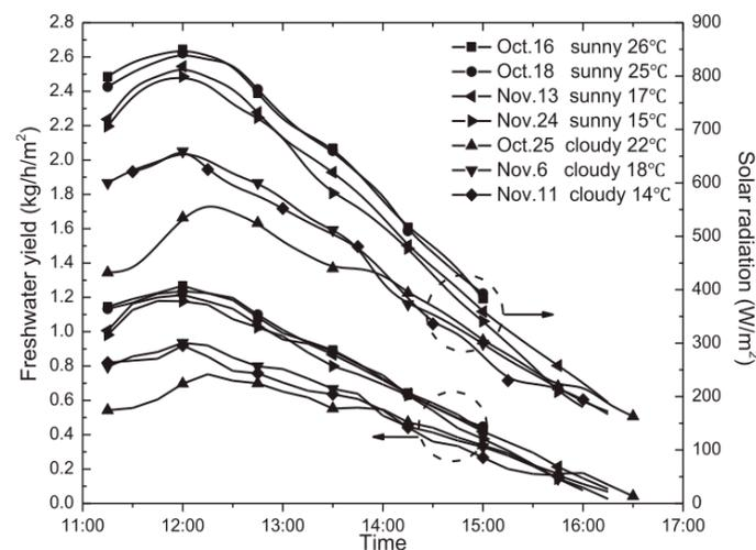
Figure 15. Clean water produced in 5 test days [52] (License Number: 5374110560616).
