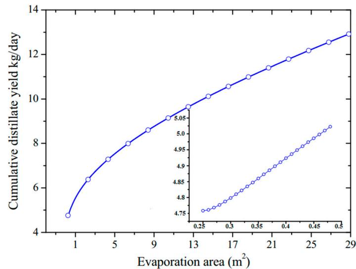
**Figure 23.** Impact of the increased evaporation size on distillation yield (stage 1) with a primary studied interval [61] (License Number: 5374100438125).
