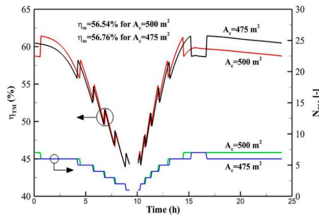
**Figure 16.** Typical daily thermal performance of the entire components used at each time ( $\eta_{TM}$ ) and the total number of working units at each time for a continuous 24 h/day process at the 475 m<sup>2</sup> and 500 m<sup>2</sup> collector size and a reservoir volume of 19 m<sup>3</sup> in October [53] (License Number: 5373840183630).
