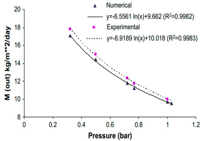
Figure 7. Difference in the still efficiency against inlet pressure [46] (License Number: 5374110080306).
