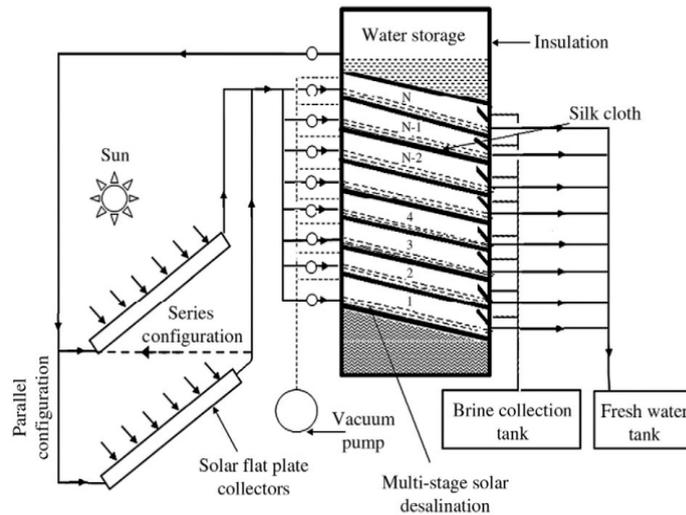
Figure 10. Multiple-stage evacuated solar distillation unit combined with flat surface collectors [48] (License Number: 5373821246523).
