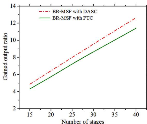
**Figure 6.** Difference of gain output ratio (GOR) with stage number for PTC-based and DASC-based BR-MSF distillation units [45] (License Number: 5374110867353).
