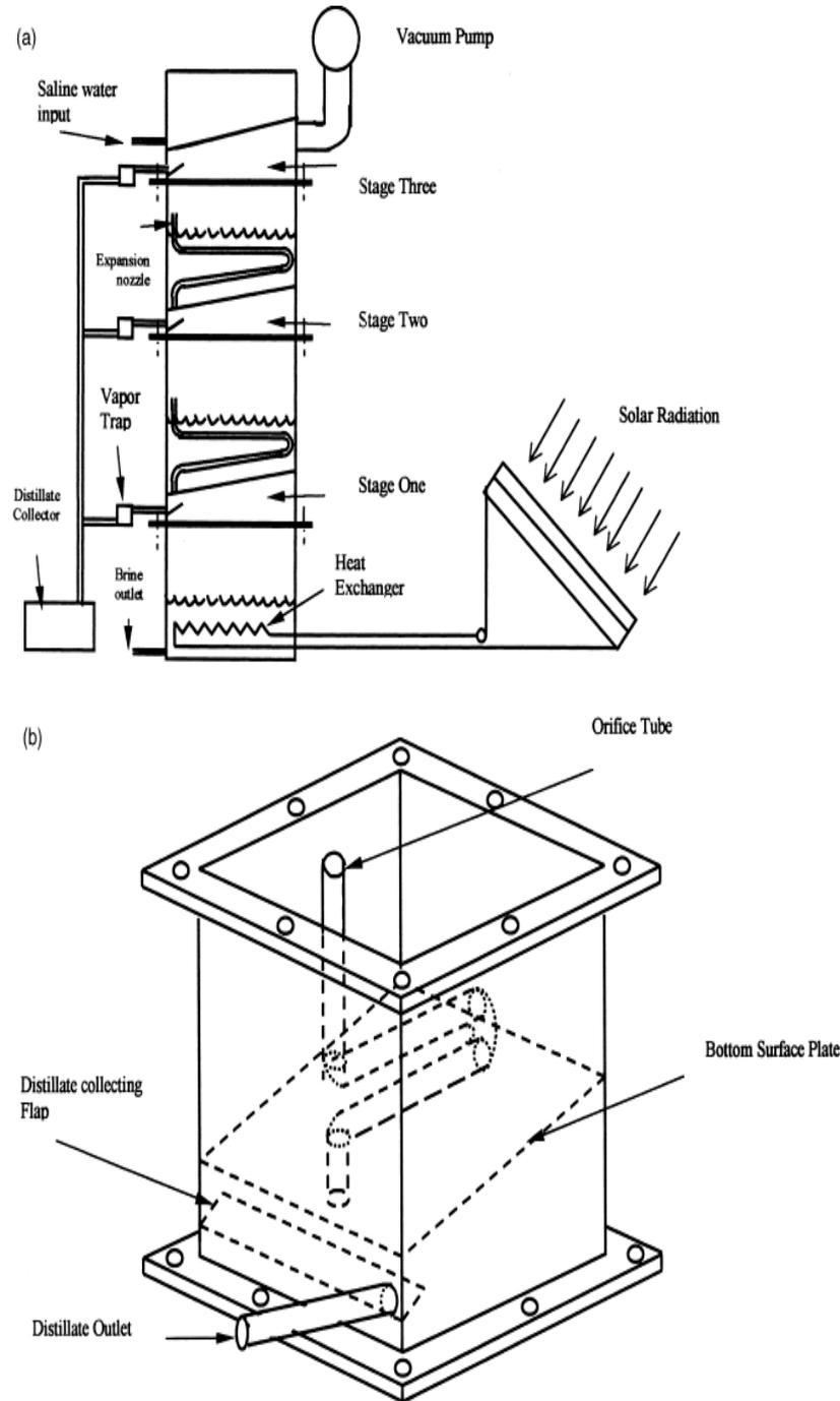
**Figure 12.** (a) Graph of the multiple-stage evacuated pack solar still. (b) Isometric view of one middle pack [50] (License Number: 5373790205227).
