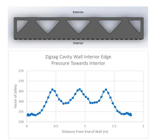
Figure 21. Results for Interior Edge of Zigzag Cavity Wall After Applying Pressure to the Interior.
