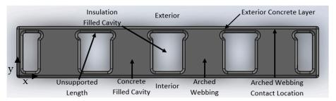
**Figure 7.** Internal Large-Arched Multicavity Wall Printed Formwork Model with Concrete Labeled. Modeled in reference to [22,30].
