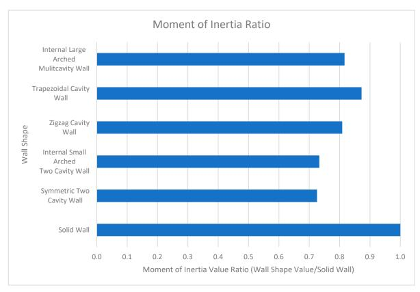
Figure 32. Moment of Inertia Ratio Chart.
