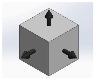
Figure 2. Three Principal Stresses on a Cube Element.
