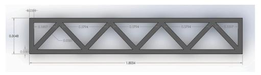
Figure 13. Zigzag Cavity Wall Printed Formwork Model. Modeled in reference to [27,28].
