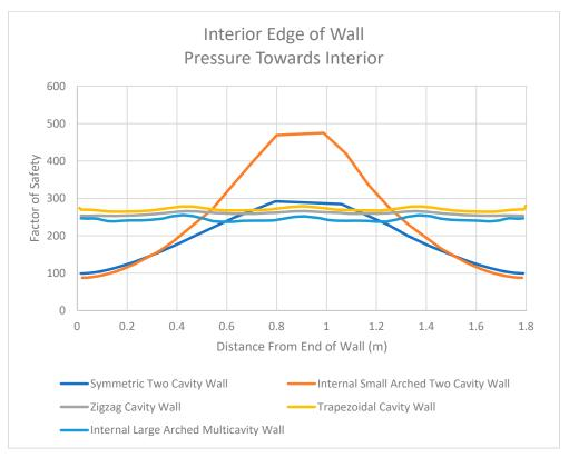
**Figure 35.** Factor of Safety Values for Interior Edge of Walls in the Midplane When Pressure Is Directed Towards the Interior.
