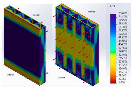
**Figure 22.** Zigzag Cavity Wall Structural Study Isometric Results for Pressure Applied Away from the Interior.
