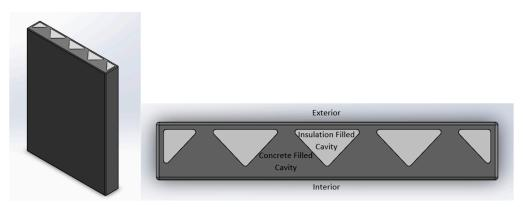
Figure 28. Zigzag Cavity Wall Concrete and Insulation Assembly.
