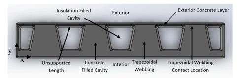
**Figure 6.** Trapezoidal Cavity Wall Printed Formwork Model with Fillets and Labels. Modeled in reference to [29].
