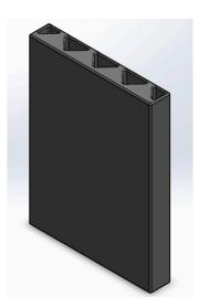
Figure 14. Zigzag Cavity Wall Printed Formwork with Interior Cavity Filled with Concrete.
