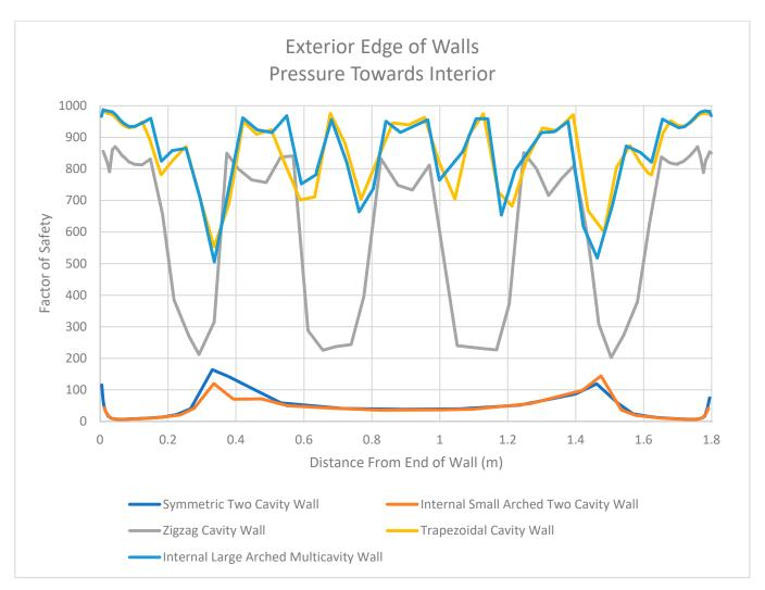
**Figure 33.** Factor of Safety Values for Exterior Edge of Walls in the Midplane When Pressure Is Directed Towards the Interior.
