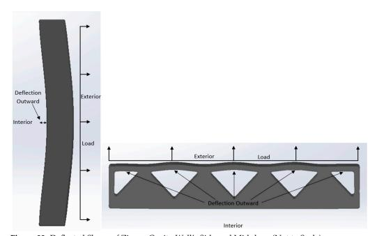
Figure 23. Deflected Shape of Zigzag Cavity Wall's Side and Midplane (Not to Scale).
