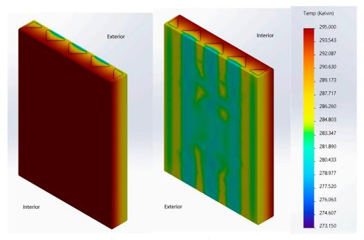
Figure 29. Zigzag Cavity Wall Isometric Temperature Plot.
