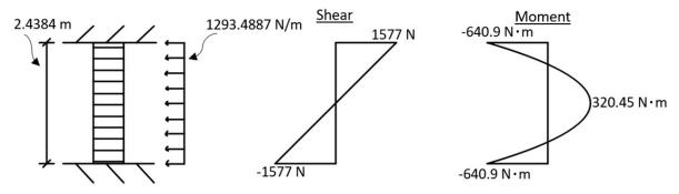
Figure 10. Loading and Moment and Shear Diagrams for Wind Loading Conditions.
