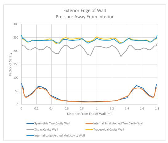
**Figure 36.** Factor of Safety Values for Exterior Edge of Walls in the Midplane When Pressure Is Directed Away from the Interior.
