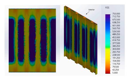
**Figure 18.** Zigzag Cavity Wall Exterior Concrete Layer Results After Applying Pressure to the Interior. Left: Exterior Side of Exterior Concrete Layer; Middle: Interior Side of Exterior Concrete Layer; Right: Color Scale of Results.
