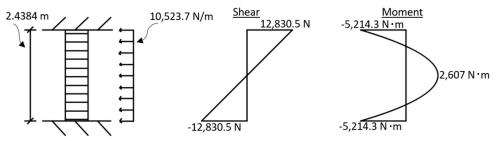
Figure 11. Loading and Moment and Shear Diagrams for Conditions in New York City, New York.
