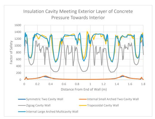
**Figure 34.** Factor of Safety Values for Insulation Cavity Meeting Exterior Layer of Concrete in the Midplane When Pressure Is Directed Towards the Interior.
