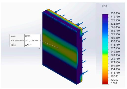
Figure 9. Factor of Safety Plot of a Solid Concrete Wall.
