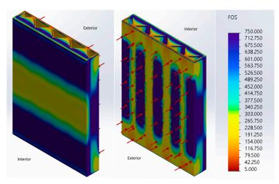
Figure 16. Zigzag Cavity Wall Structural Study Isometric Results After Applying Pressure to the Interior.
