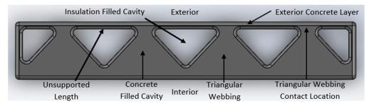
Figure 15. Zigzag Cavity Wall Printed Formwork Filled with Concrete, Labeled.
