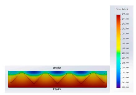
Figure 30. Zigzag Cavity Wall Overhead Temperature Plot.
