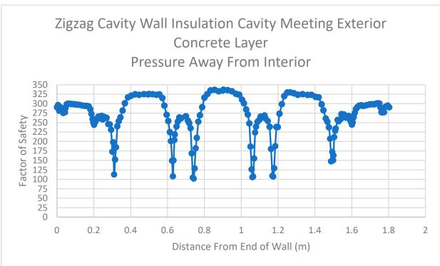
**Figure 26.** Results for Insulation Cavity Meeting the Exterior Concrete Layer of the Zigzag Cavity Wall for Pressure Applied Away from the Interior.
