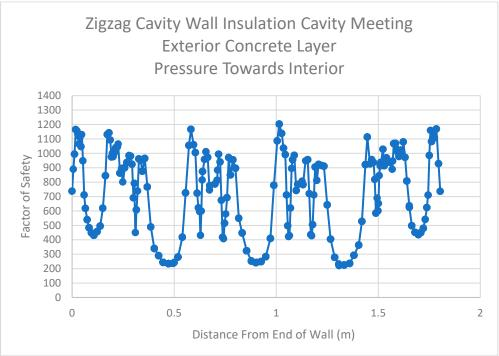
**Figure 20.** Results for Insulation Cavity Meeting the Exterior Concrete Layer of the Zigzag Cavity Wall After Applying Pressure to the Interior.
