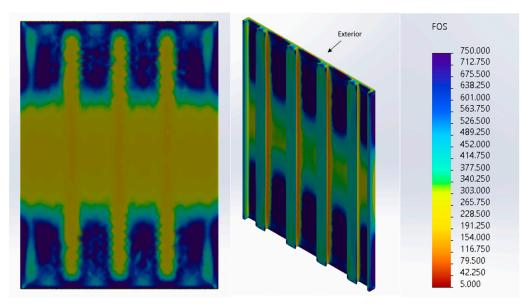
**Figure 24.** Zigzag Cavity Wall Exterior Concrete Layer Results for Pressure Applied Away from the Interior. Left: Exterior Side of Exterior Concrete Layer; Middle: Interior Side of Exterior Concrete Layer; Right: Color Scale of Results.
