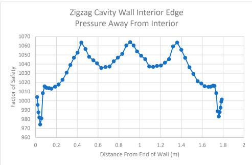
Figure 27. Zigzag Cavity Wall Interior Edge Results for Pressure Applied Away from the Interior.
