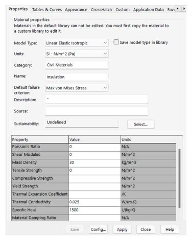
Figure 8. Creation of Insulation Material Properties.
