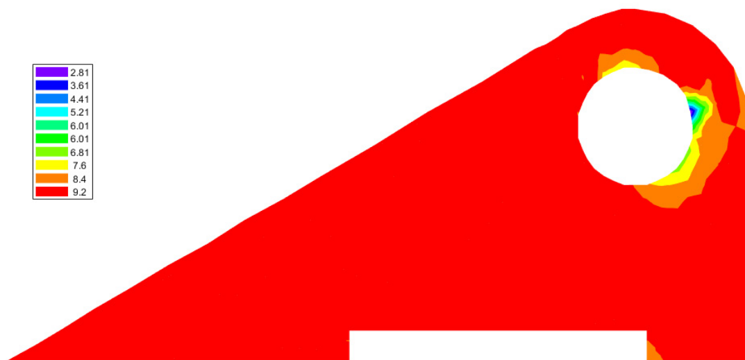
Figure 5. Reliability index distribution of the stresses in the initial mooring bracket.
