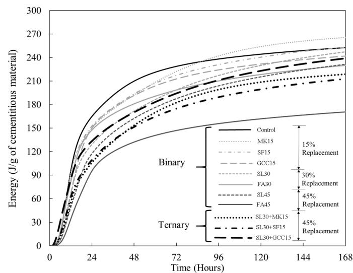
**Figure 7.** Heat of hydration of binary and ternary mixtures including ground calcium carbonate (GCC) in the 422 group.
