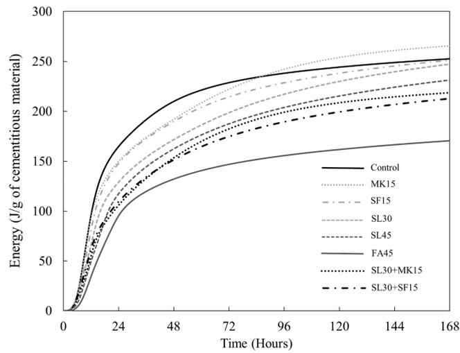
Figure 10. Heat of hydration of the 422 group mixtures to generate pozzolanic reaction.
