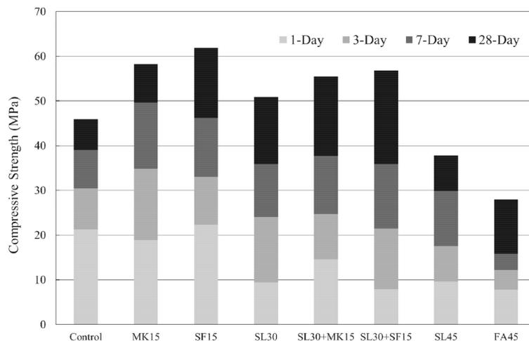
Figure 6. Compressive strength development of the 422 group mixtures.
