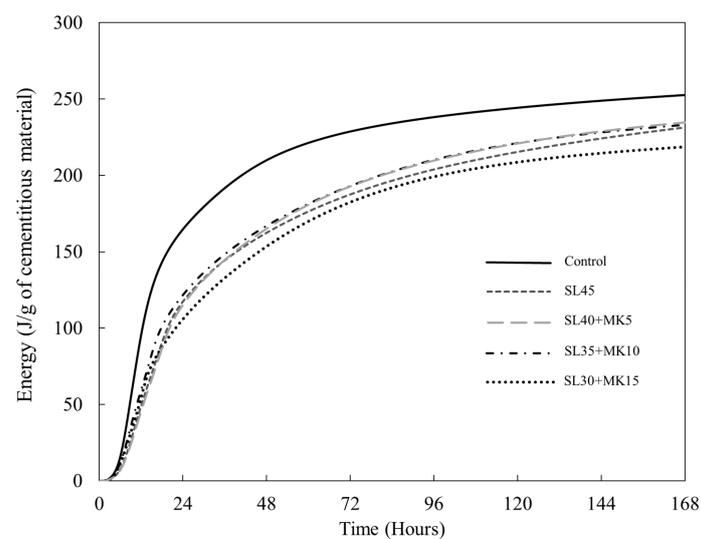
**Figure 8.** Heat of hydration of binary and ternary mixtures including slag (SL) and metakaolin (MK) in the 422 group.
