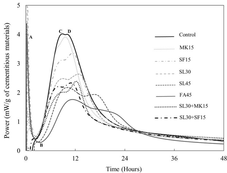
Figure 4. Rate of heat flow of 422 group mixtures.
