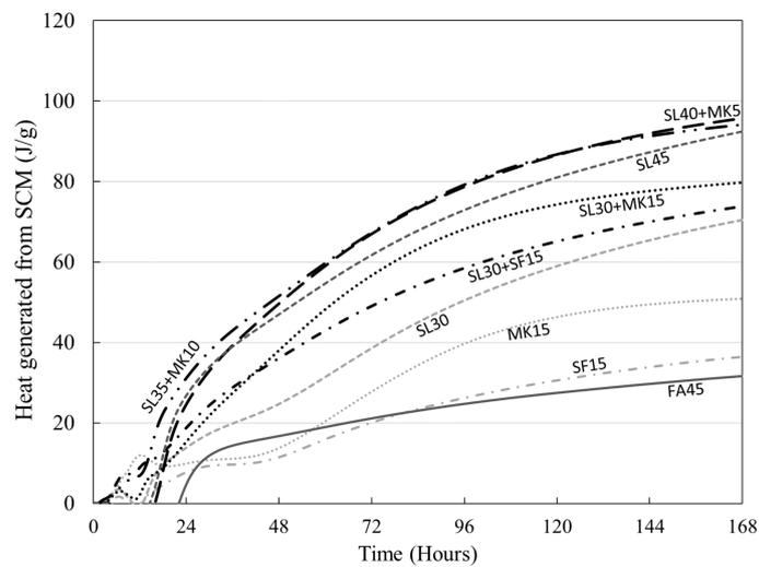
Figure 11. Heat of hydration generated from the pozzolanic reaction.
