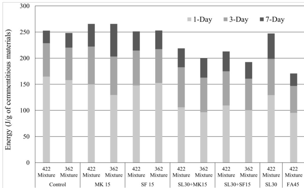
Figure 2. Heat of hydration of 422 and 363 mixture groups.
