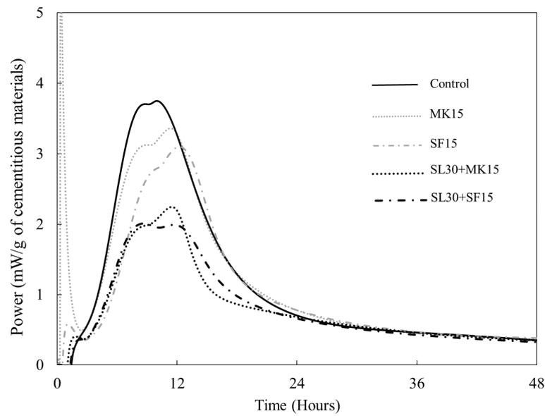
Figure 3. Rate of heat flow of 363 group mixtures.
