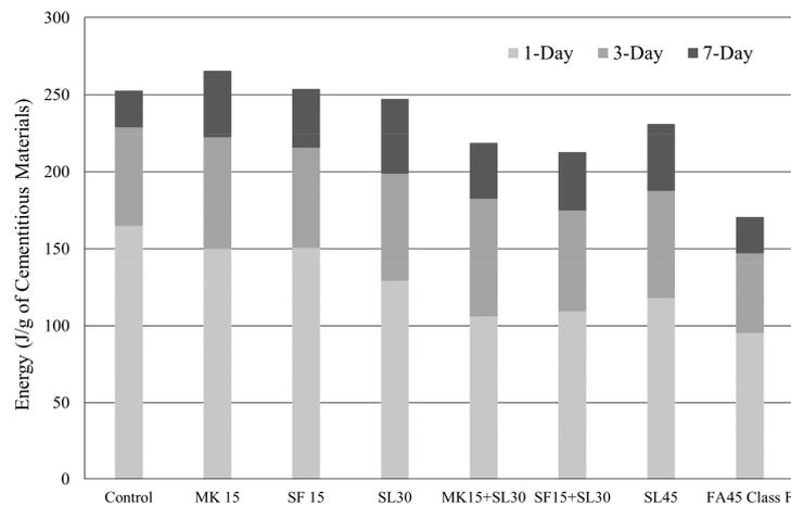
Figure 5. Heat of hydration of the 422 group mixtures.
