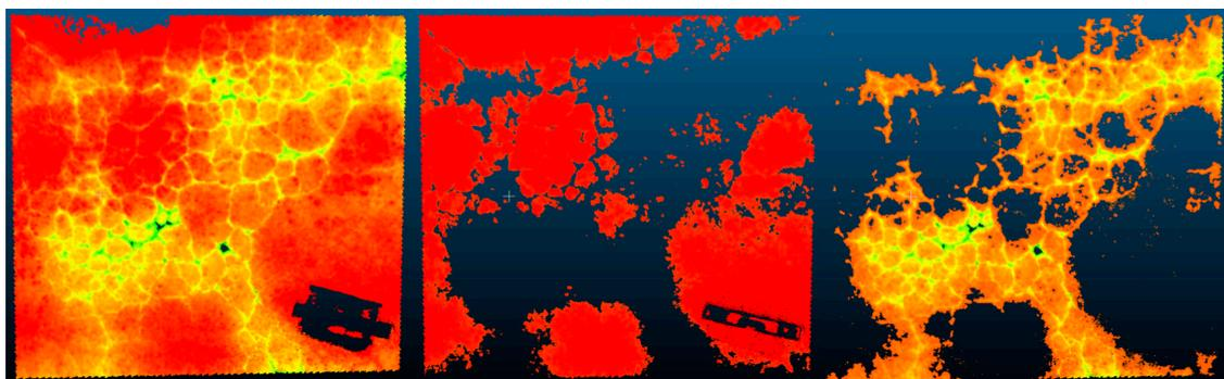
Figure 27. Segmentation of pavement section 3 with RANSAC.
