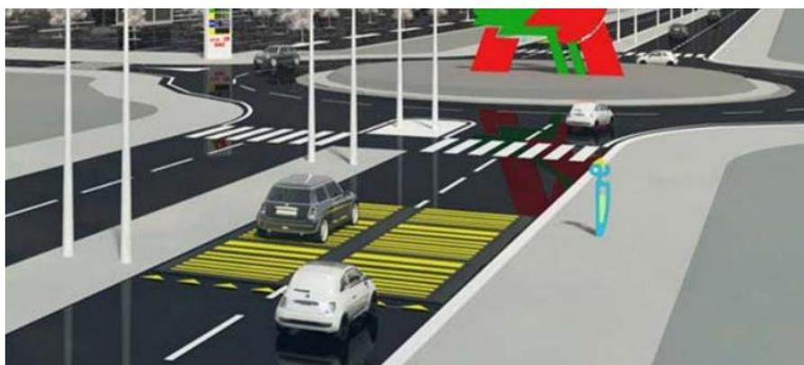
**Figure 2.** Artificial road roughness system for battery roads [8].
