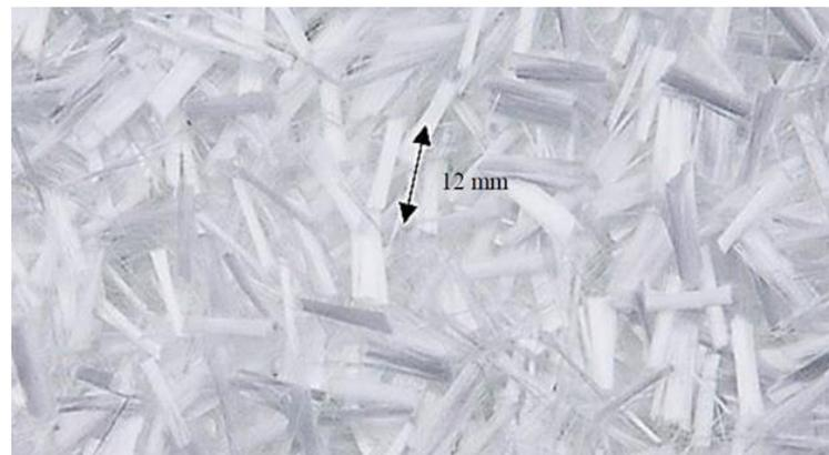
**Figure 1.** Monofilament micro-synthetic fibers.
