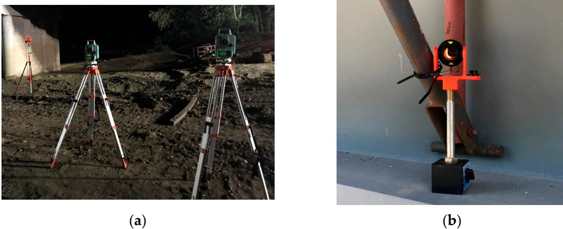
**Figure 11.** Total station and prism: (a) Total station. (b) Prism.
