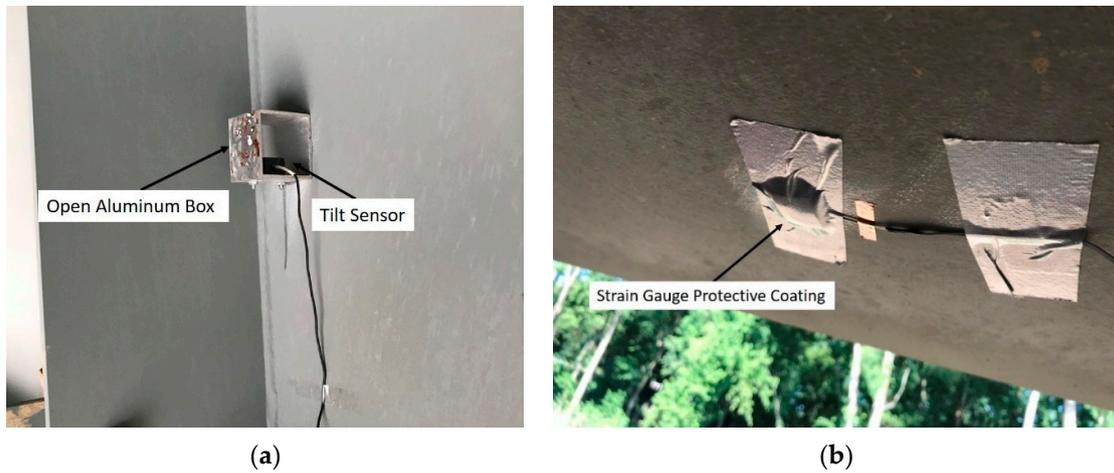
**Figure 10.** Tilt sensor and strain gauge: (a) Tilt sensor with open aluminum box. (b) Strain gauge with protective coating.
