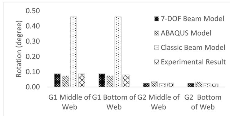
Figure 21. Rotation comparison among different numerical models and experimental data for S1 section.
