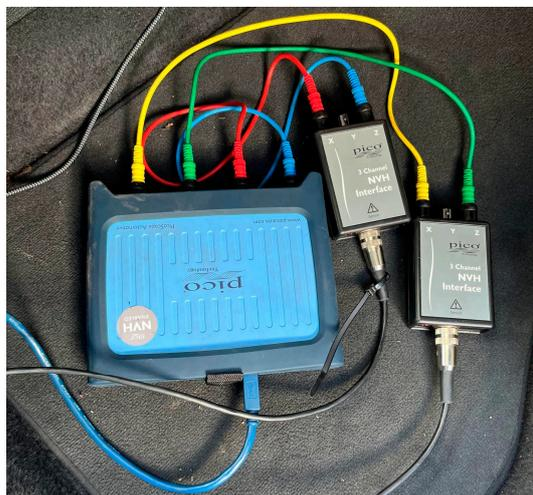
**Figure 4.** The measurement system, including the attenuators and the scope.
