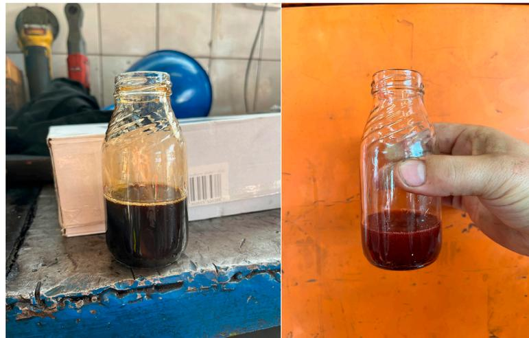
**Figure 1.** The automatic transmission fluid before and after the oil change.
