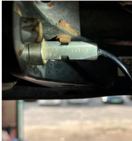
**Figure 3.** The location of the accelerometer on the bracket.
