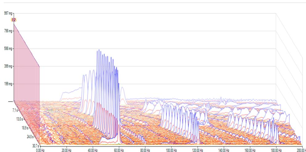
Figure 11. Vibrations in the frequency domain before the oil change, 0–70 km/h.
