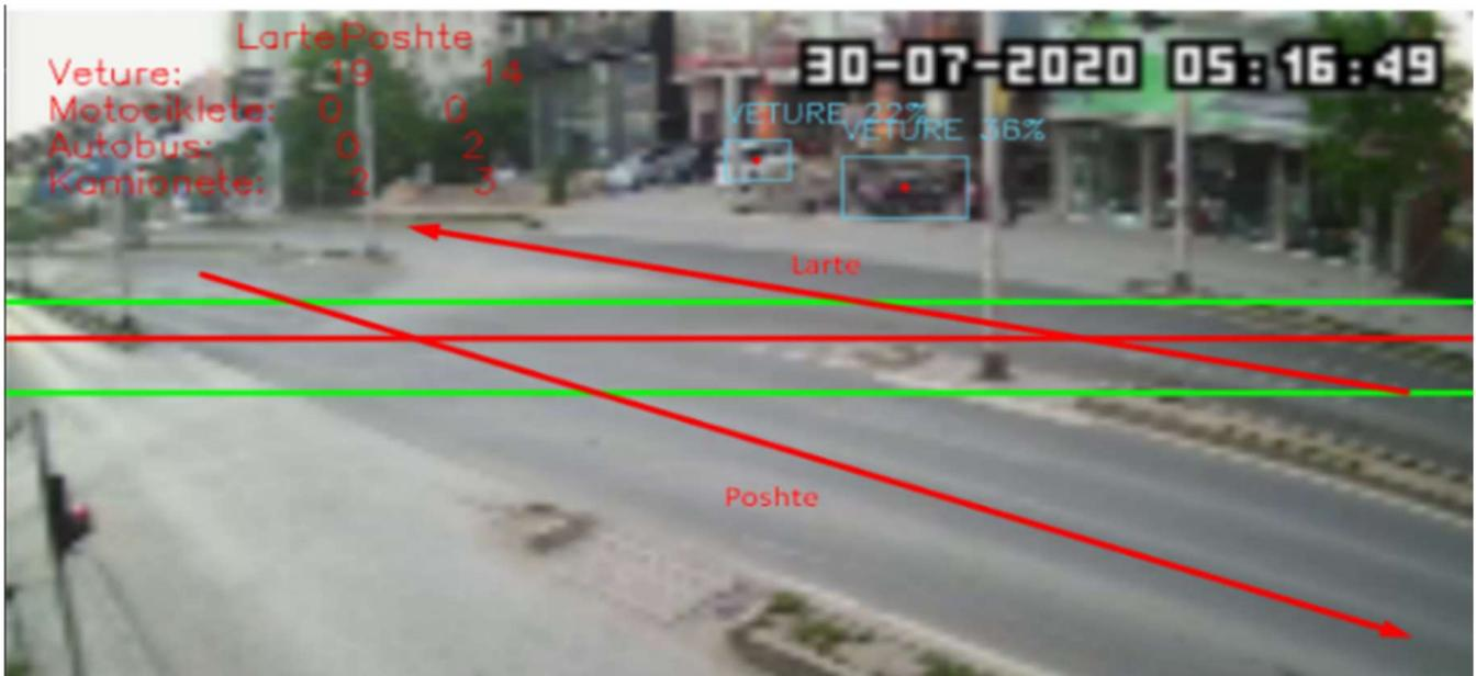
**Figure 4.** Traffic count from camera and data processing in program (05:00–05:15).
