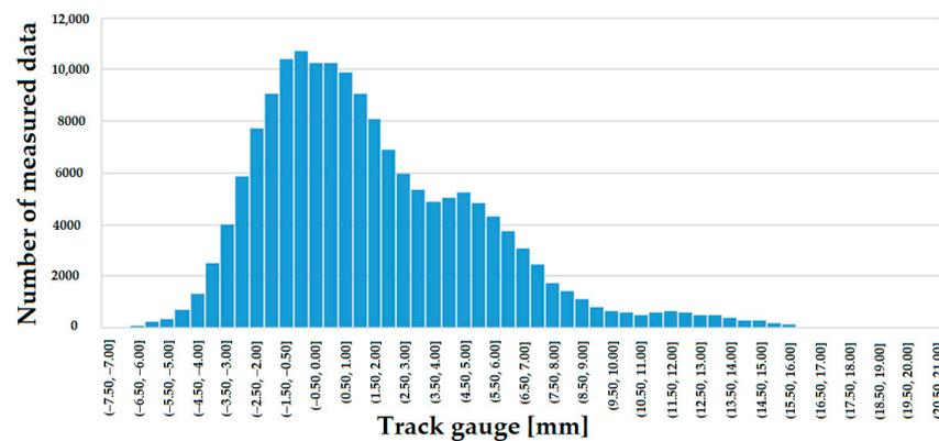
Figure 13. Probability density function of track gauge parameter on Line #1, circular curves (CCs).
