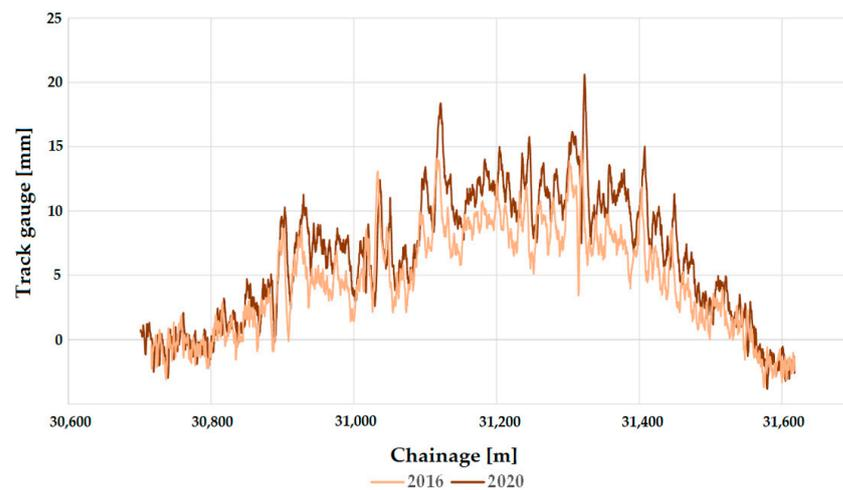
**Figure 19.** The longitudinal function of the track gauge on Line #1 (between Biatorbágy and Herceghalom railway stations), considering the measurement data in 2016 and 2020 and the sections with ECs.
