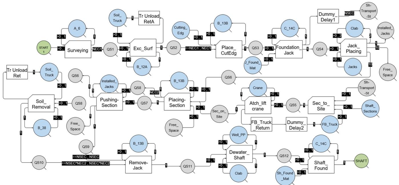
Figure 2. Shaft construction sequence using the segmental method.
