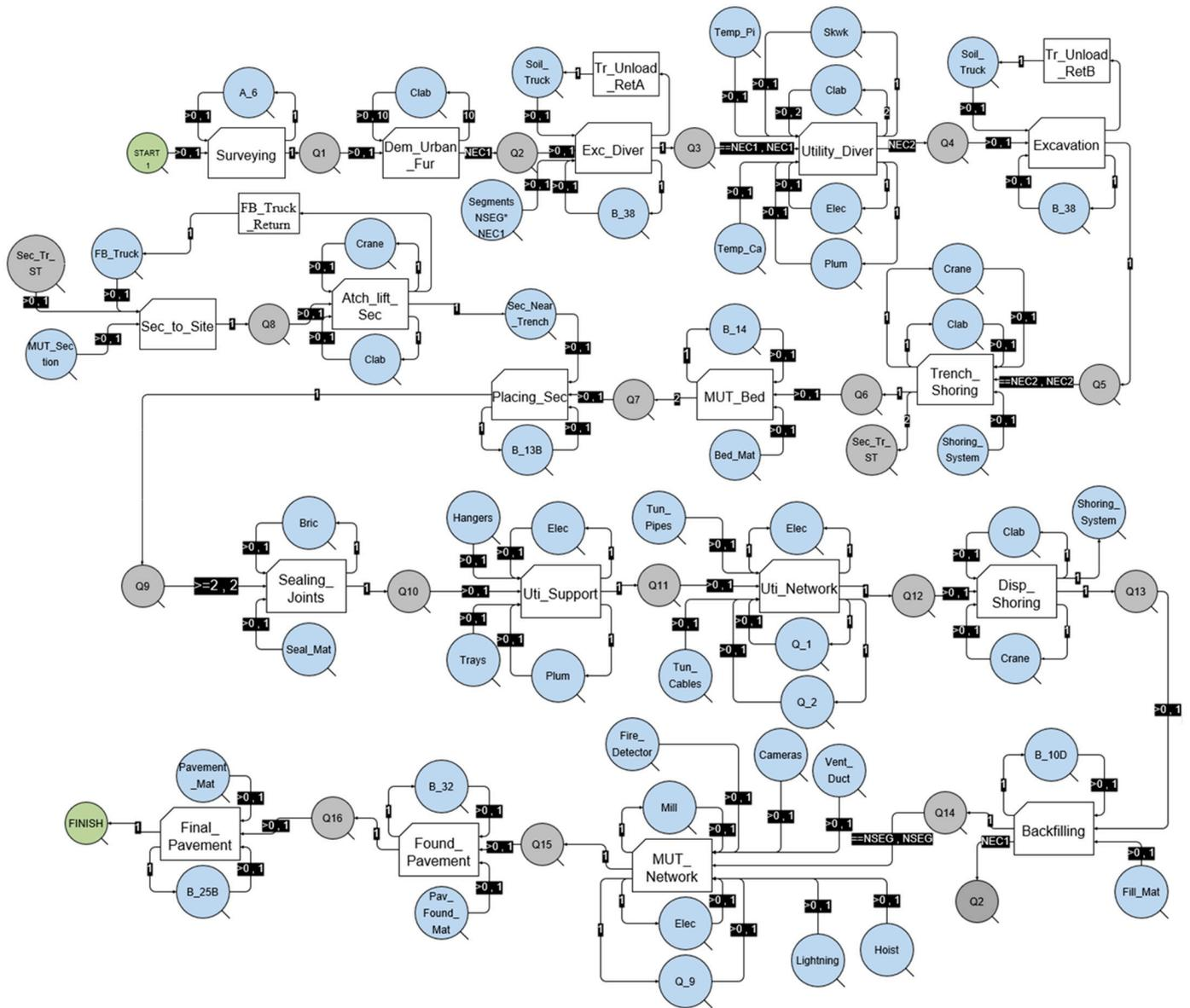
Figure 1. MUT construction sequence using C&C method.
