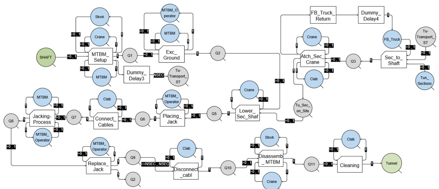
Figure 3. Tunnel construction sequence in microtunneling method.
