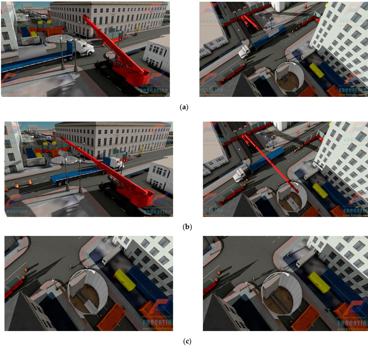
**Figure 9.** Four-dimensional simulation of MUT construction using microtunneling in Fuzor 2022 software: (a) delivering tunnel section to the construction site; (b) lifting and placing the section into the starting shaft; and (c) pushing the section into the ground.
