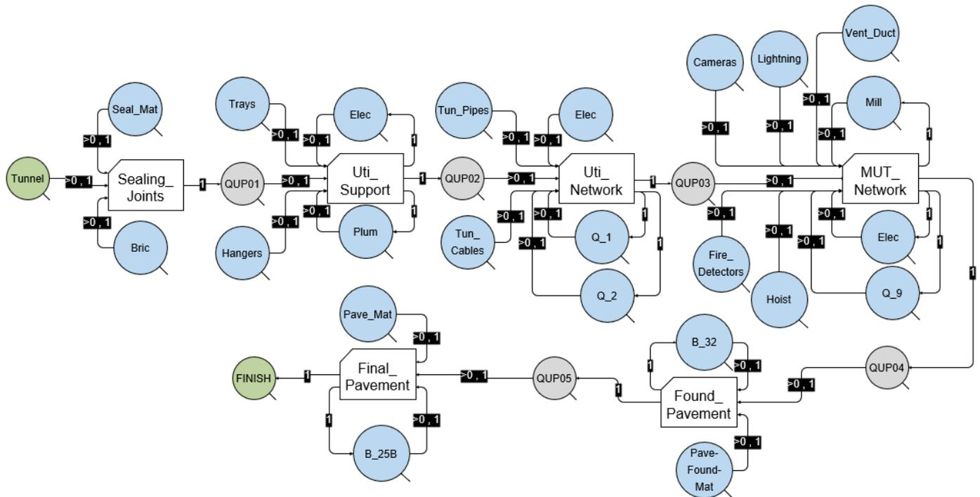
Figure 4. Construction sequence for placing utilities in the tunnel.
