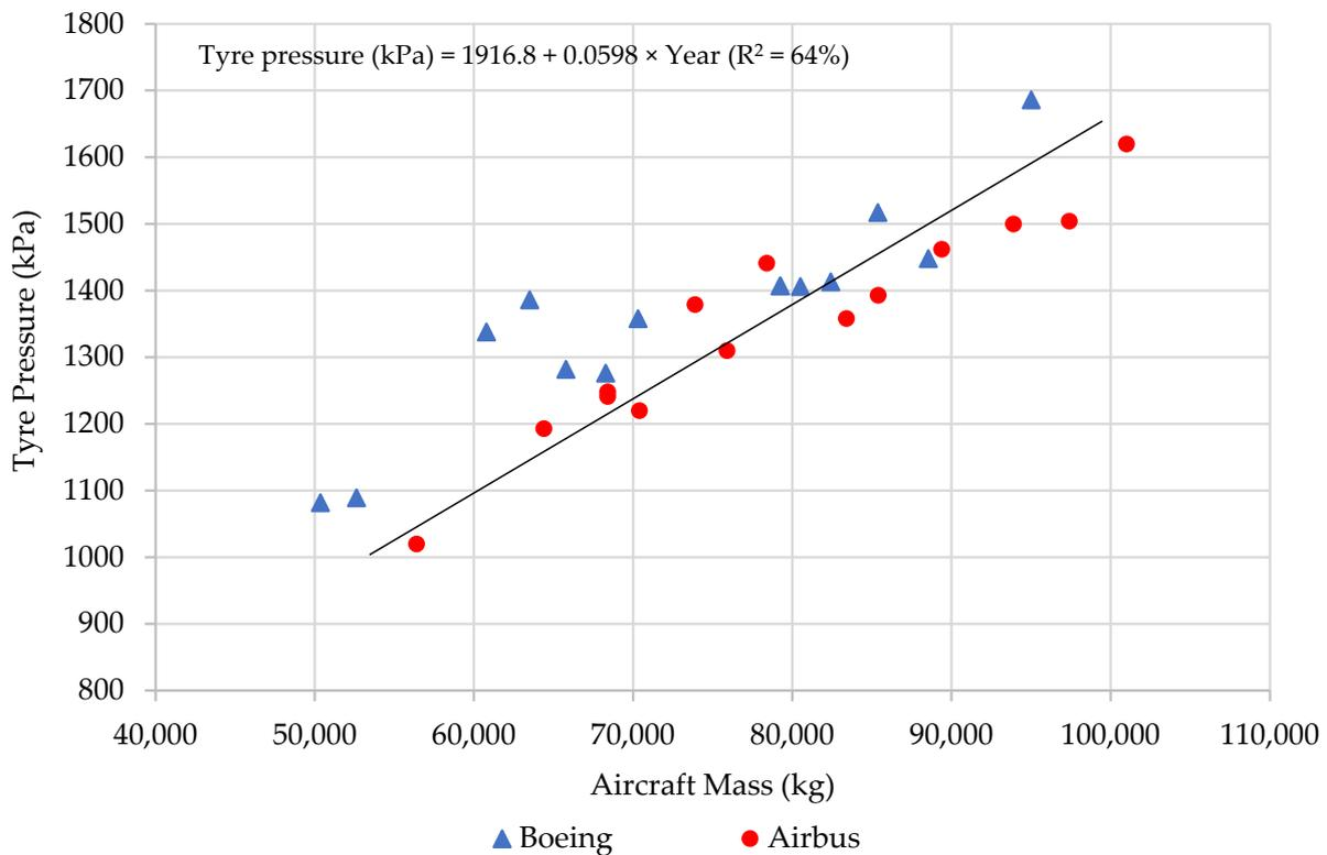
Figure 4. Aircraft tyre pressure increases with aircraft weight increases.
