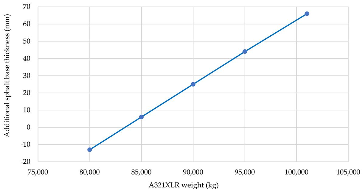
**Figure 9.** Additional asphalt thickness as a function of A321XLR operating weight.
