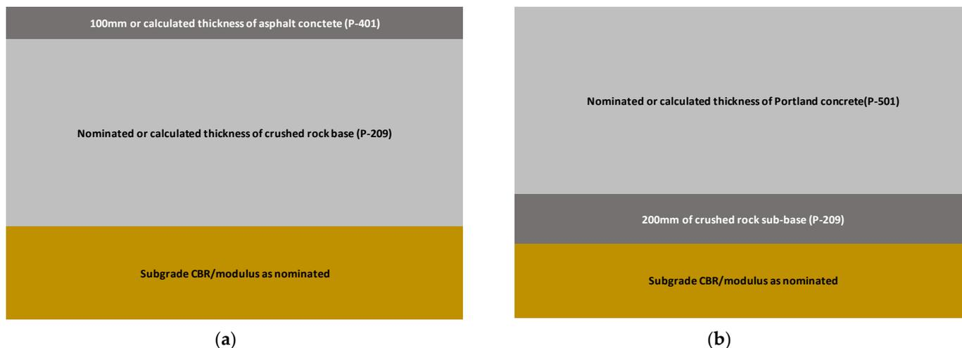
**Figure 2.** Schematic (a) flexible and (b) rigid pavement compositions.
