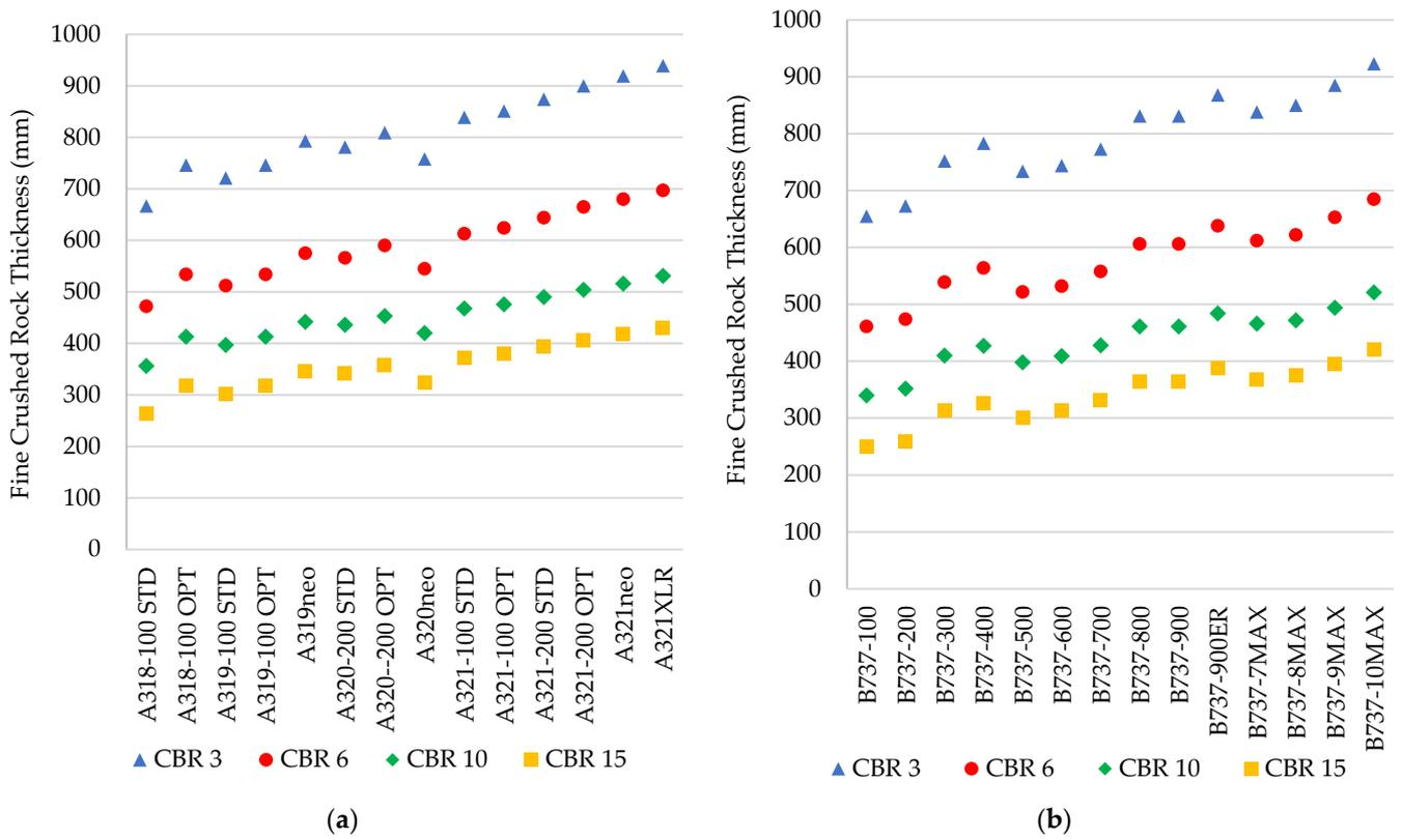
Figure 7. Flexible pavement thicknesses for (a) A320 and (b) B737 aircraft.
