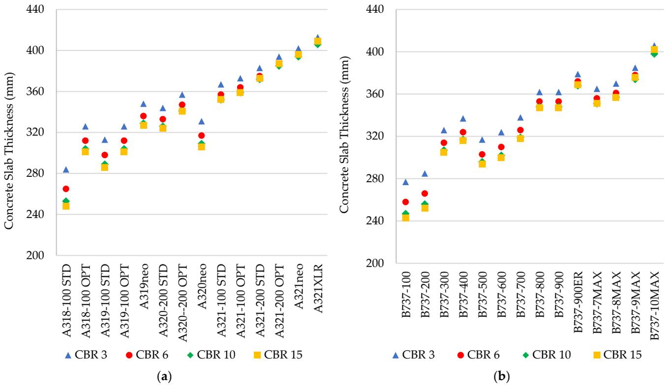
Figure 8. Rigid pavement thicknesses for (a) A320 and (b) B737 aircraft.
