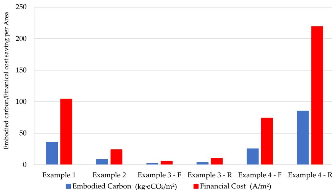
**Figure 11.** Relative embodied carbon and financial cost savings. Note: R and F indicate the flexible and rigid pavements where both pavement types were considered for the sample example airport.
