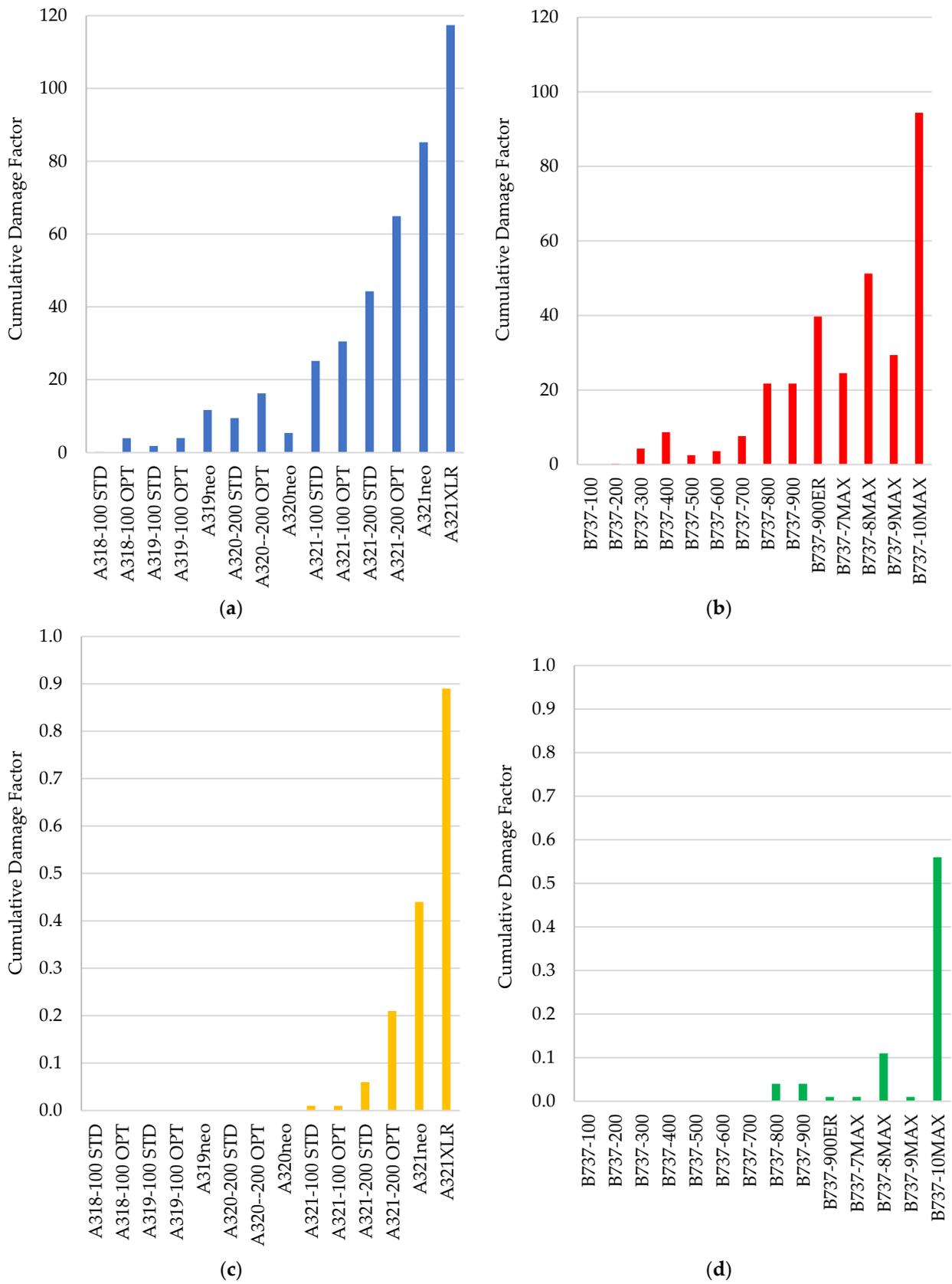
**Figure 5.** Effect of aircraft variant on fixed flexible pavement thickness for (a) A320 on thin pavement, (b) B737 on thin pavement, (c) A320 on thick pavement and (d) B737 on thick pavement.
