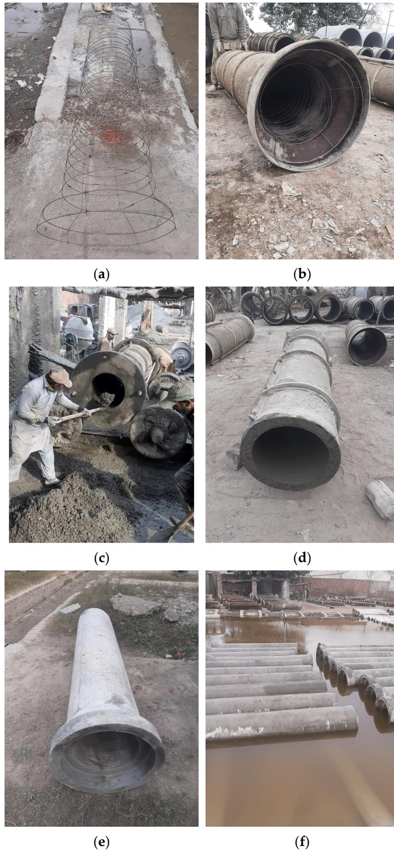
**Figure 2.** Pipe casting procedure; (a) steel fixing; (b) mold preparation with steel cage; (c) feeding concrete; (d) filled pipe in mold; (e) demolded concrete pipe; (f) pipe curing.
