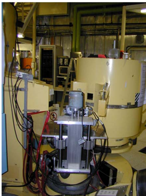
Figure 5. The Triple Axis Strain Scanner at HIFAR 2004. Australian Centre for Neutron Scattering Photograph archives; © ANSTO used with permission.
