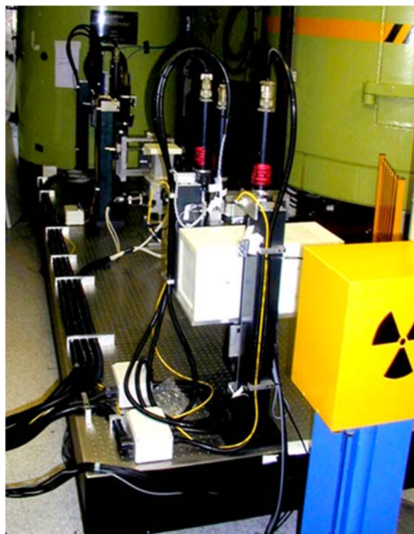
Figure 4. Neutron Reflectometer at HIFAR 2004. Australian Centre for Neutron Scattering Photograph archives; © ANSTO used with permission.
