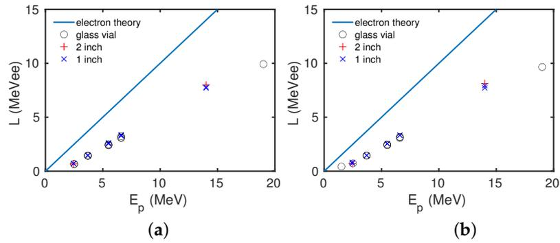
**Figure 3.** Light output function for all measurements detected using (a) PYR5/DIPN scintillator, (b) THIO5/DIPN scintillator.
