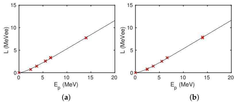
**Figure 4.** Light output function for all measurements detected using a 1 inch (a) PYR5/DIPN scintillator, and (b) THIO5/DIPN scintillator. The data points are completed with fit functions for each scintillator. The fit functions are described in Table 1.
