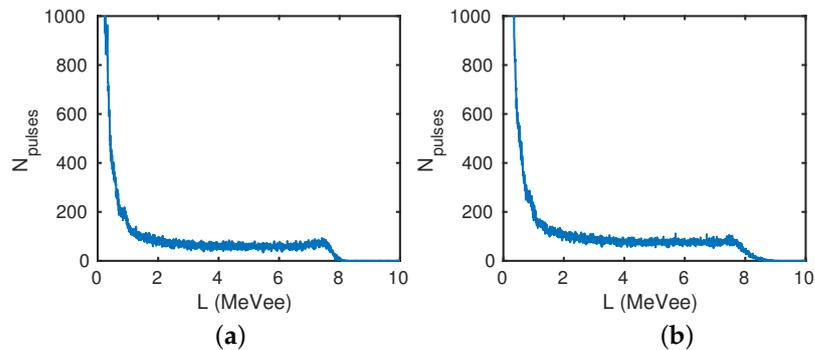
**Figure 2.** The number of pulses detected as a function of the equivalent electron energy  $L$ : (a) Neutrons from the DT reaction with an energy of  $E_n = 14$  MeV detected using 1 inch PYR5/DIPN scintillator. (b) Neutrons from the DT reaction with an energy of  $E_n = 14$  MeV detected using 1 inch THIO5/DIPN scintillator.
