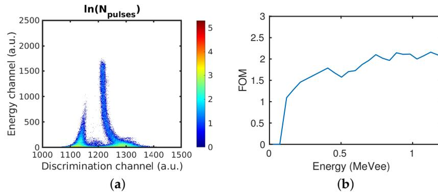
**Figure 1.** (a) Two-parameter histogram of the DT reaction with an energy of  $E_n = 14$  MeV detected using a 1 inch PYR5/DIPN scintillator. (b) FOM for the same measurement.
