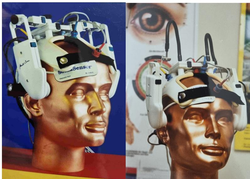
**Figure 2.** Multiparametric helmet construction in acupuncture research from 1997 (© Gerhard Litscher).
