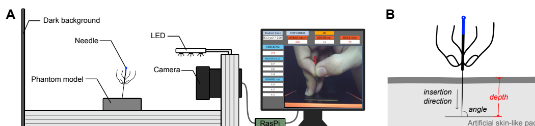
Figure 2. The vision-based needle tracking system. (A) The hardware setup. (B) Acupuncture needle manipulation parameters. In this work, we focused on the insertion depth.
