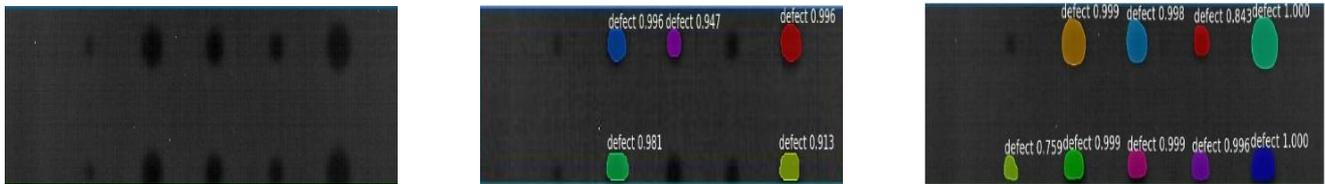
(d) Example 1 from CFRP specimen (left: ground truth; middle: training without synthetic data; right: training with synthetic data)
