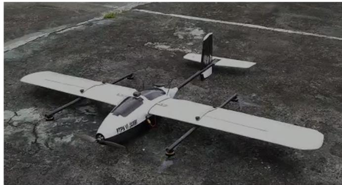
**Figure 3.** Fixed Wing VTOL drone.
