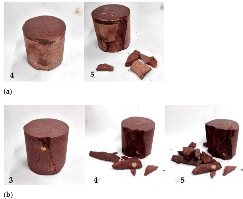
**Figure 8.** Failure form of rock samples. (a) Semisaturated sample. (b) Saturated samples.
