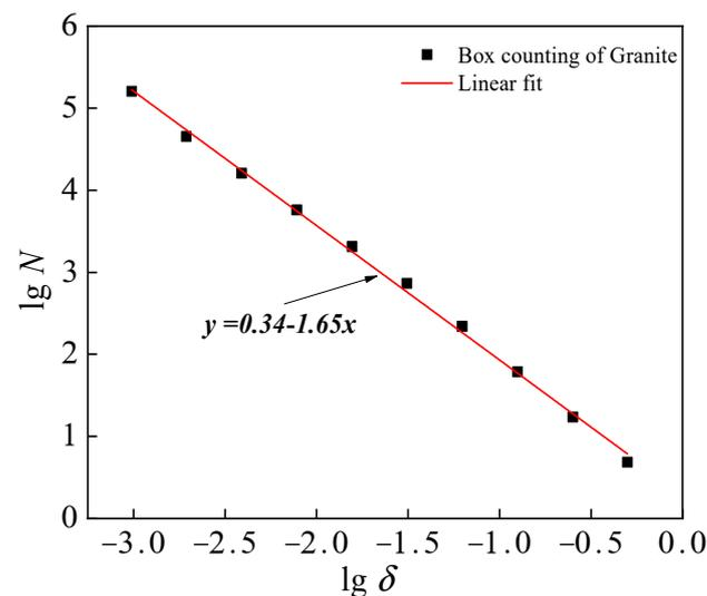
**Figure 12.** Box-counting method double logarithmic diagram for granite.
