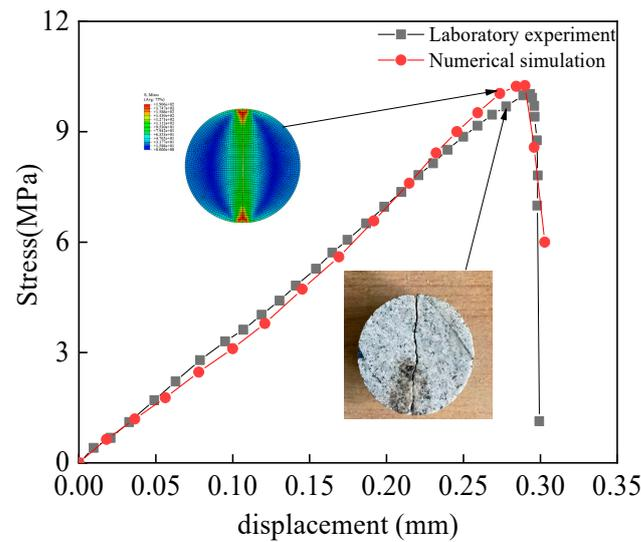
**Figure 11.** Comparisons of the stress–displacement curves measured in numerical simulation and laboratory experiments.
