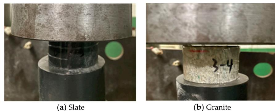
**Figure 2.** Uniaxial compression test.
