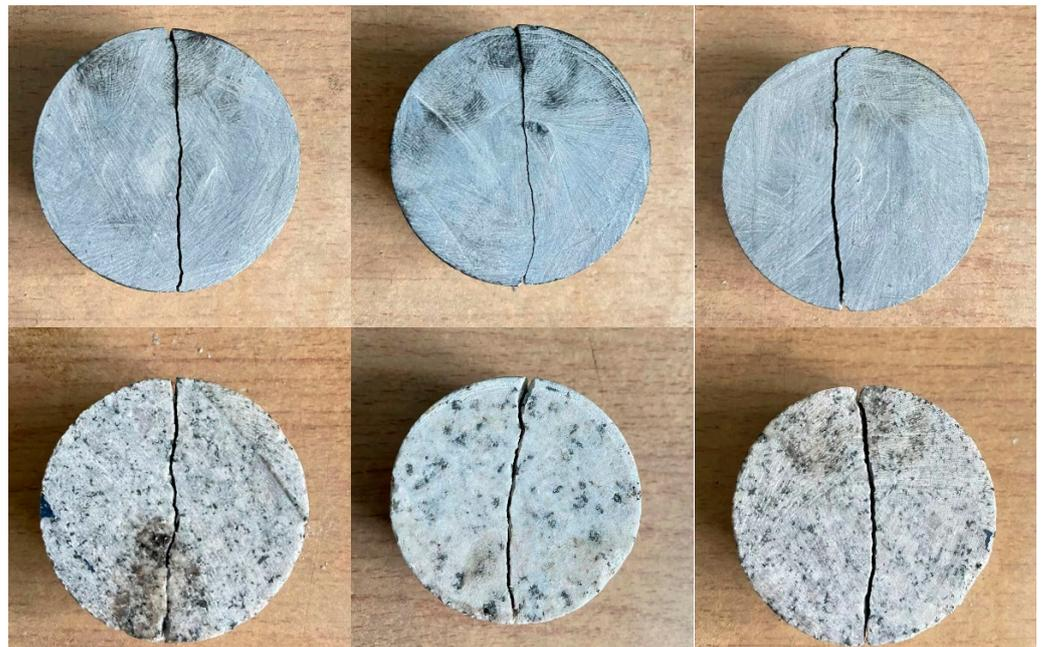
**Figure 3.** Failure patterns of some specimens under static load (slate and granite).
