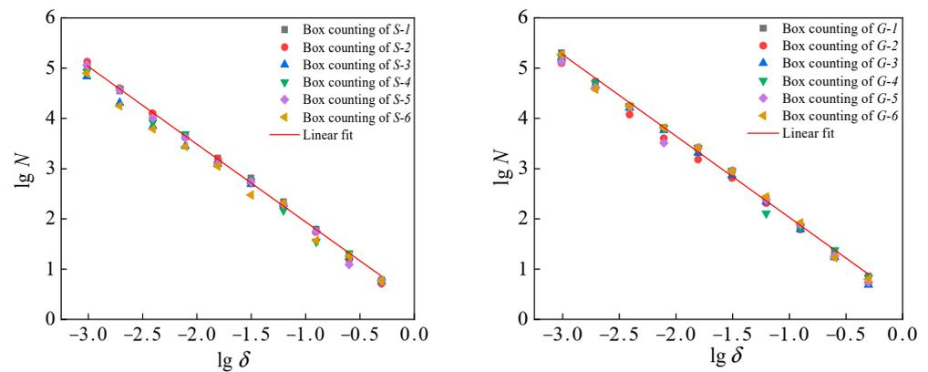
Figure 4. Box-counting method double logarithmic diagram for slate and granite.
