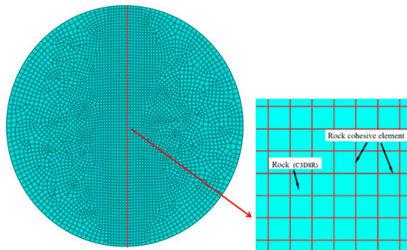
**Figure 8.** Finite element mesh.
