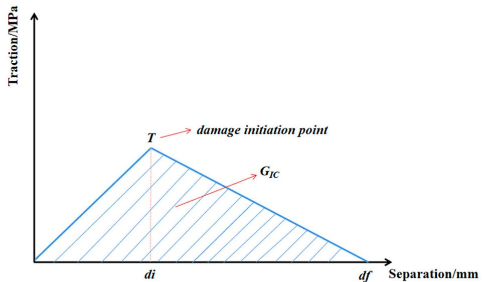
Figure 6. Cohesion model used in this paper.
