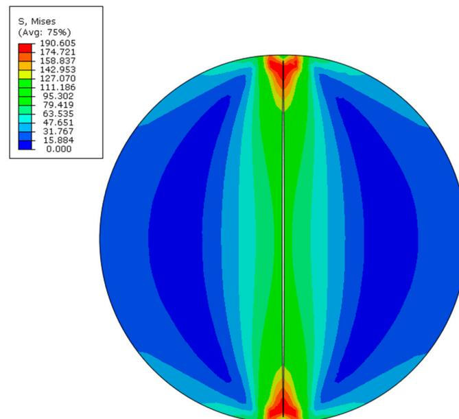
**Figure 10.** Numerical simulation of Brazilian splitting for ideal homogeneous model.
