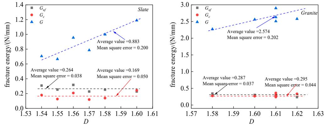
Figure 5. Three fracture energies and complexity  $D$  of slate and granite.
