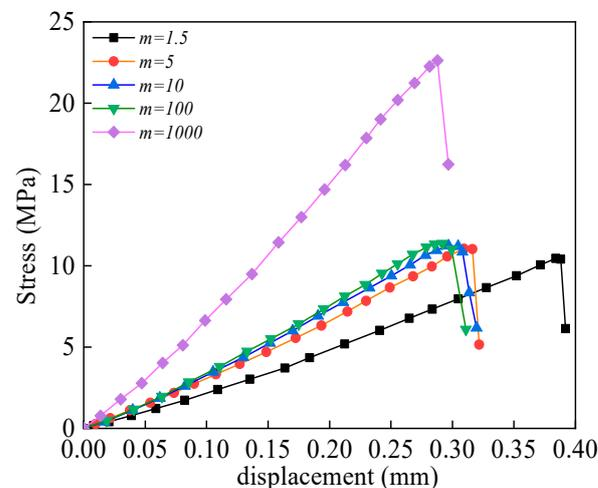
**Figure 15.** Stress–displacement curves in different homogeneity cases.
