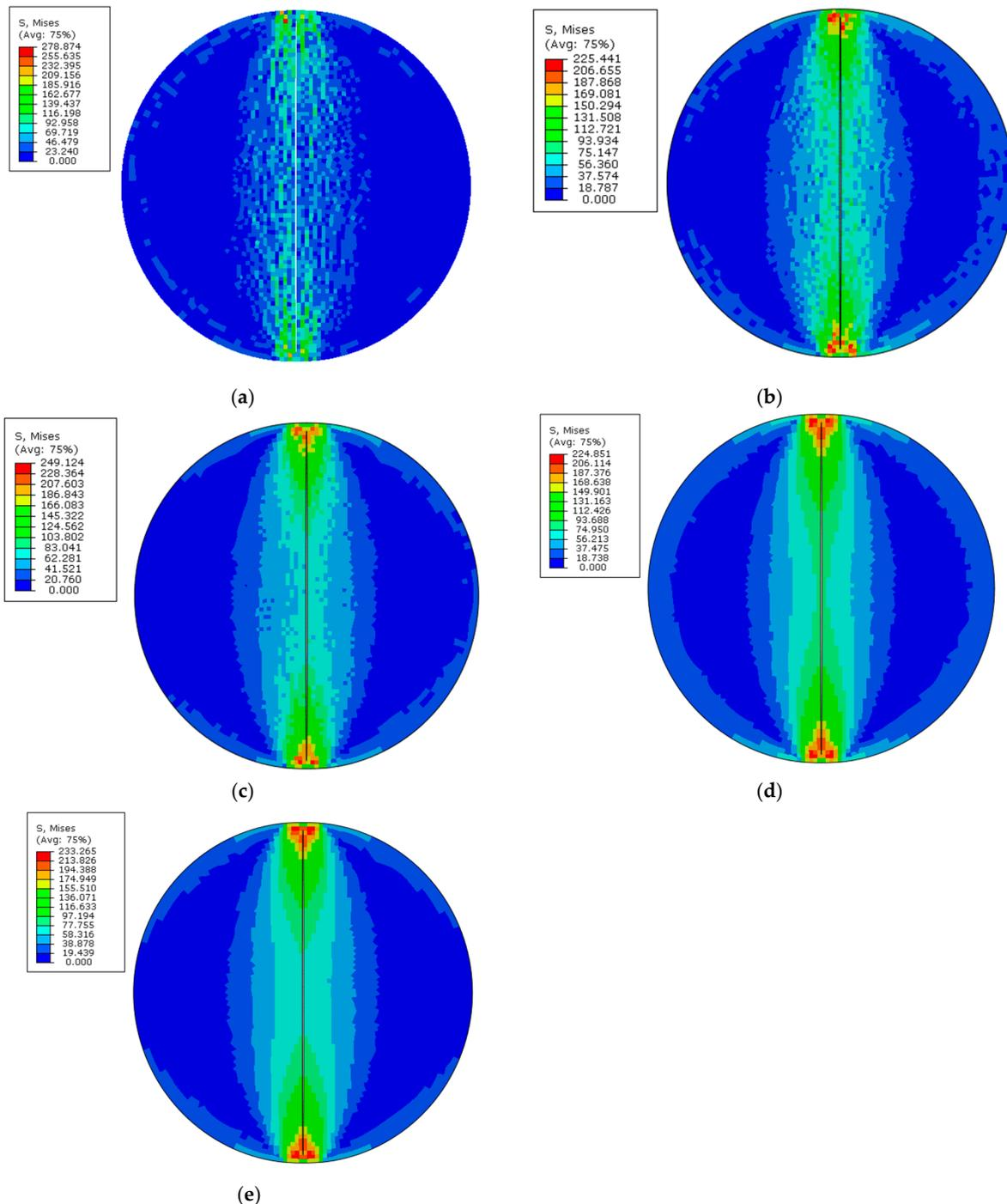
**Figure 13.** Numerical simulation of Brazilian splitting for heterogeneous model. (a)  $m = 1.5$ ; (b)  $m = 5$ ; (c)  $m = 10$ ; (d)  $m = 100$ ; (e)  $m = 1000$ .
