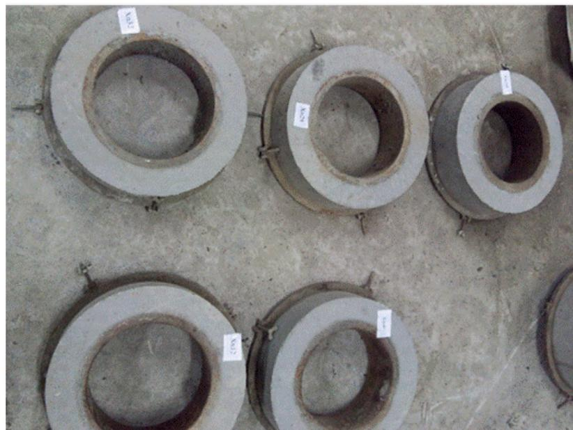
**Figure 2.** The picture of the restrained concrete ring test.
