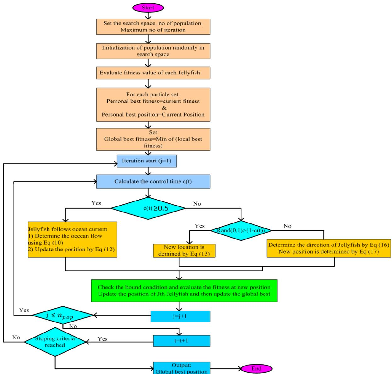
Figure 4. The Schematic flow chart for JSO.
