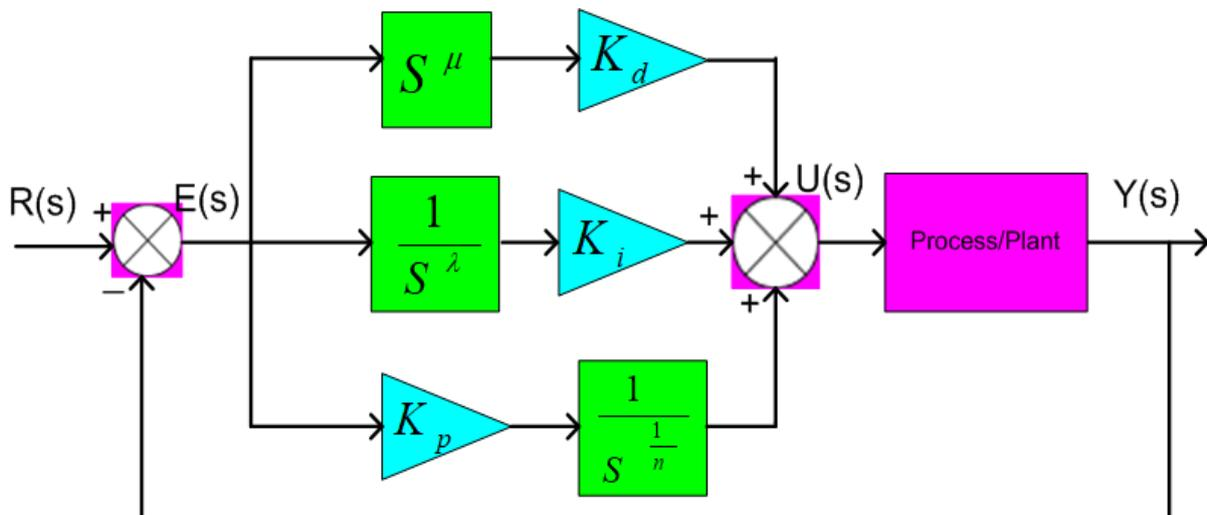
Figure 5. Structure of FOPID controller.
