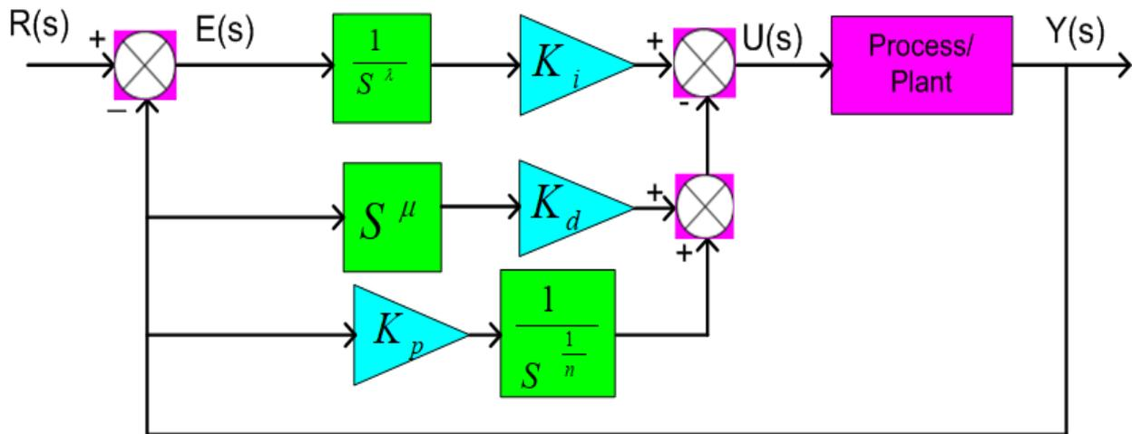
Figure 6. Structure of MFOPID controller.
