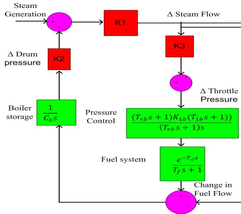
Figure 2. Schematic model of boiler dynamic.
