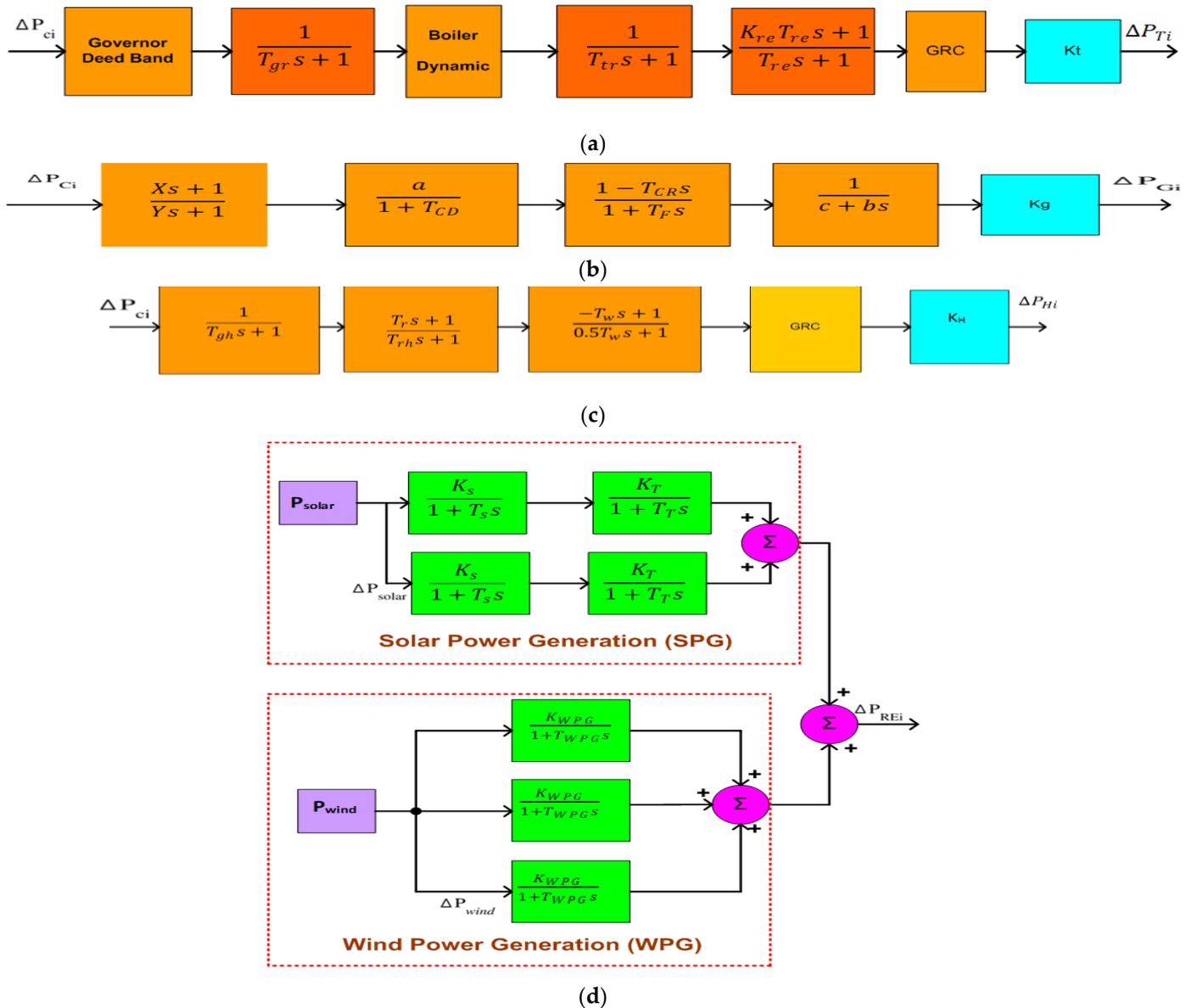
Figure 3. TF model for; (a) reheat thermal, (b) gas, (c) hydro, (d) RES.
