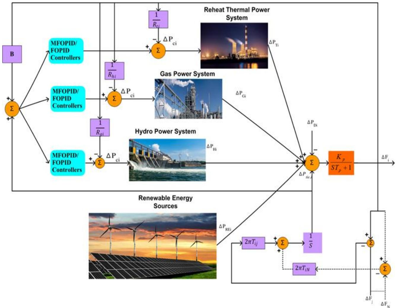
Figure 1. Schematic diagram of proposed power system.
