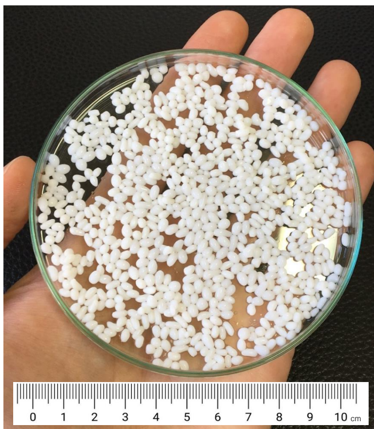
Figure S1. Zn-Al- ^{15}\text{NO}_3 layered double hydroxides encapsulated in alginate beads (LDH-AN).
