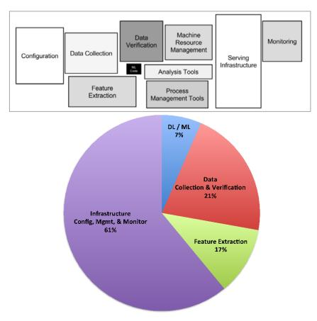
Figure 5. The hidden technical debt in machine learning systems (adapted from [6]).
