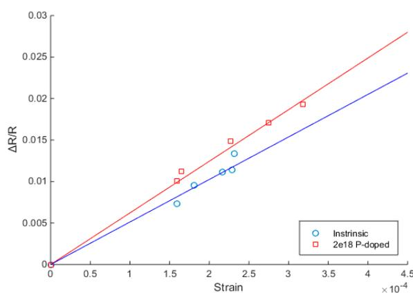
**Figure 4.** Change in resistance against strain.
