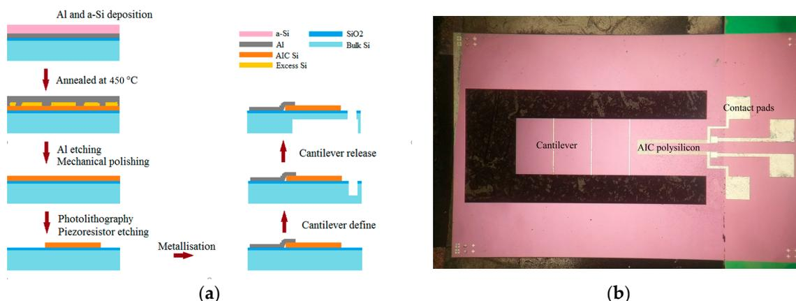
**Figure 1.** (a) Fabrication process of AIC polysilicon and the test structure; (b) Optical image of the cantilever with polysilicon on top.
