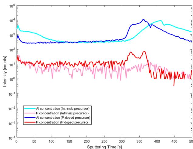
**Figure 2.** TF-SIMS measurement of doped AIC polysilicon.
