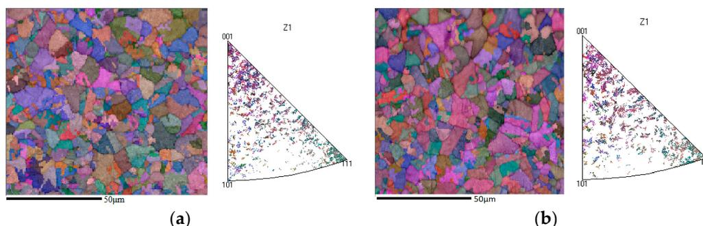
**Figure 3.** (a) EBSD of intrinsic precursor; (b) EBSD of  $2 \times 10^{18}/\text{cm}^3$  phosphorus doped precursor.
