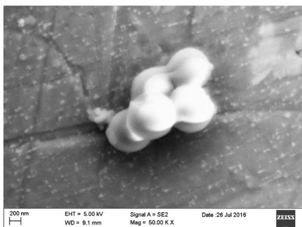
**Figure 2.** SEM image of corrole-polyacrolein. The diameter of each microsphere is of the order of few hundreds of nanometers.
