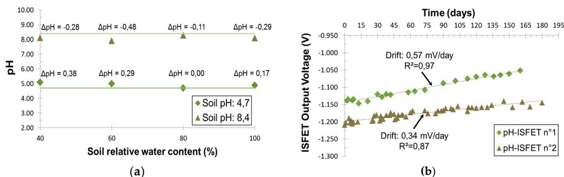
**Figure 2.** (a) Comparison of pH measurements performed by pH-ISFET at different soil moisture levels in an acid and a basic silty-clay soil. The difference with the standard method of soil pH determination (green lines) is indicated above each measurement point; (b) Time evolution of the output voltage of two pH-ISFET inserted in a silty-clay soil for six months.
