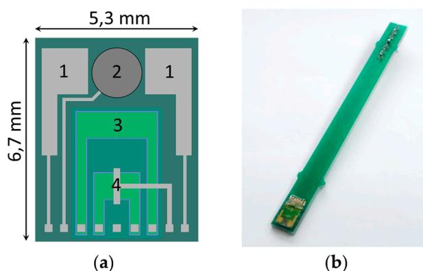
**Figure 1.** (a) Schematic top view of the microsystem. (1) Platinum electrodes for EC measurements; (2) Miniature Ag/AgCl quasi-reference electrode; (3) ISFET micro-sensor; (4) MOSFET for temperature measurement; (b) View of the chip after electronic packaging on a printed-circuit board (PCB) and encapsulation.
