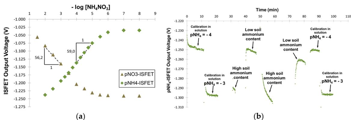
**Figure 3.** (a) Calibration curves of the  $\text{pNO}_3^-$ -ISFET and  $\text{pNH}_4^+$ -ISFET in aqueous solution of  $\text{NH}_4\text{NO}_3$ ; (b) Plot vs. Time of  $\text{pNH}_4^+$ -ISFET signal. The measurements are first done in two calibration solutions, and then in high and low nitrogen content soils before being checked again in the two same calibration solutions.
