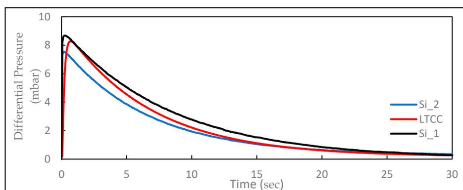
Figure 4. Experimental differential pressure data once the heater is switch off, Gas: Nitrogen.
