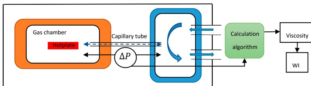
Figure 1. Schematic of the sensor and its working principle.
