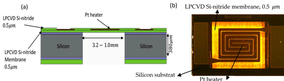
Figure 3. (a) Schematic cross-section of various layers comprising a Silicon micro-hotplate; (b) Fabricated micro-hotplate, Si<sub>1</sub>-top side view.
