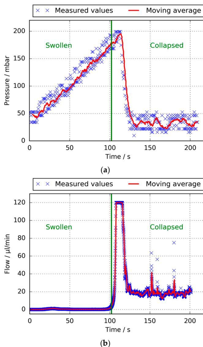
**Figure 2.** Proof-of-concept for the application as microvalve: Pressure (a) and flow (b) within the system for the swollen and collapsed state of the hydrogel, the green line indicates the power-on event of the stimulus. For the swollen hydrogel, the channel is blocked so that no significant flow occurs and the pressure rises. When the hydrogel collapses, the channel is opened leading to a decrease in pressure and the liquid flows through the microfluidic.
