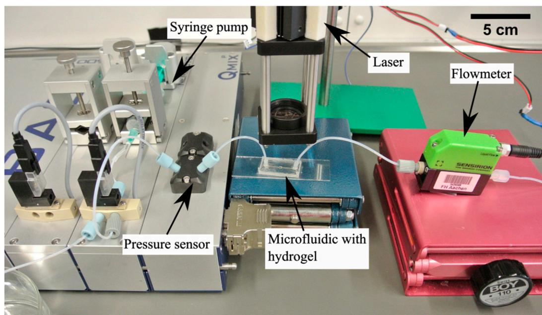
**Figure 1.** Setup for the characterization of the valve functionality including a laser for the stimulation of the hydrogels, a syringe pump to generate the required flow and a pressure sensor and a flowmeter to record the relevant parameters within the system.
