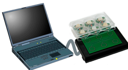
Figure 2. Wireless electronic readout system carrying a standard 6 well titer plate equipped with 6 NFC tags [3] to perform the impedance measurement of the sensors.
