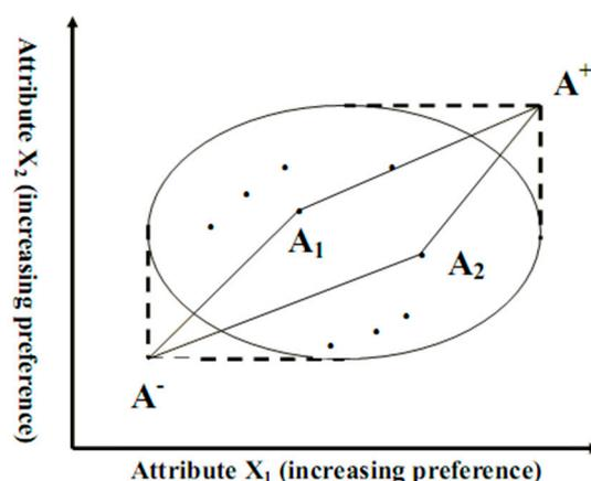
**Figure 1.** Basic concept of TOPSIS method (A<sup>+</sup>: Ideal point, A<sup>-</sup>: Negative—Ideal Point).
