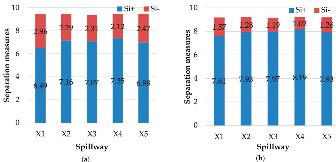
**Figure 3.** Separation measures; Ideal separation ( $S_i^+$ ). Negative-ideal separation ( $S_i^-$ ). (a) 1st approach (linear scale transformation); (b) 2nd approach (Jahanshahloo et al. formula).
