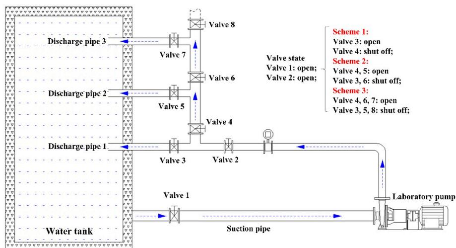
Figure 2. The test rig of three different discharge piping schemes.
