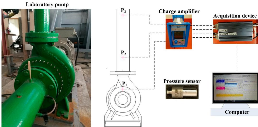
Figure 1. Schematic view of the experimental instrumentation.
