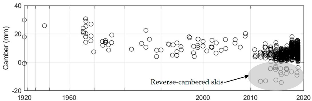
Figure 4. Maximum camber vs. model year. Negative camber represents fully-rocker (or reverse-cambered) skis.
