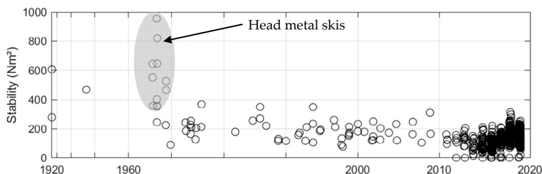
**Figure 9.** Directional stability estimated at a lateral lean angle of  $45^\circ$ .
