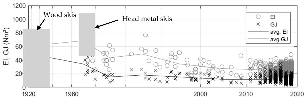
**Figure 7.** Length-averaged bending and torsional stiffnesses vs. model year. The solid lines, ‘avg. EI’ and ‘avg. GJ’ are the mean values averaged over each whole decade.
