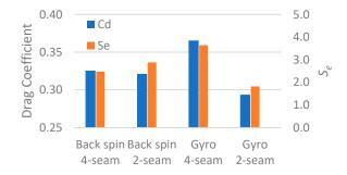
**Figure 8.** The comparison between  $S_e$  and the average drag coefficient of each spin orientation.
