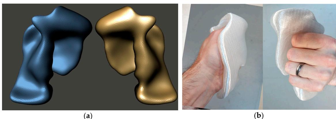
**Figure 6.** Latest design solution: (a) final CAD models of the pair of customised wheelchair racing gloves; (b) the 3D printed gloves being tested for fit using Premium PLA (Raise3D) material.
