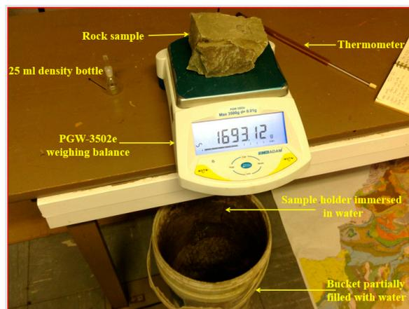
**Figure 3.** Photo demonstrating the use of Archimedes' principle in rock sample measurements.
