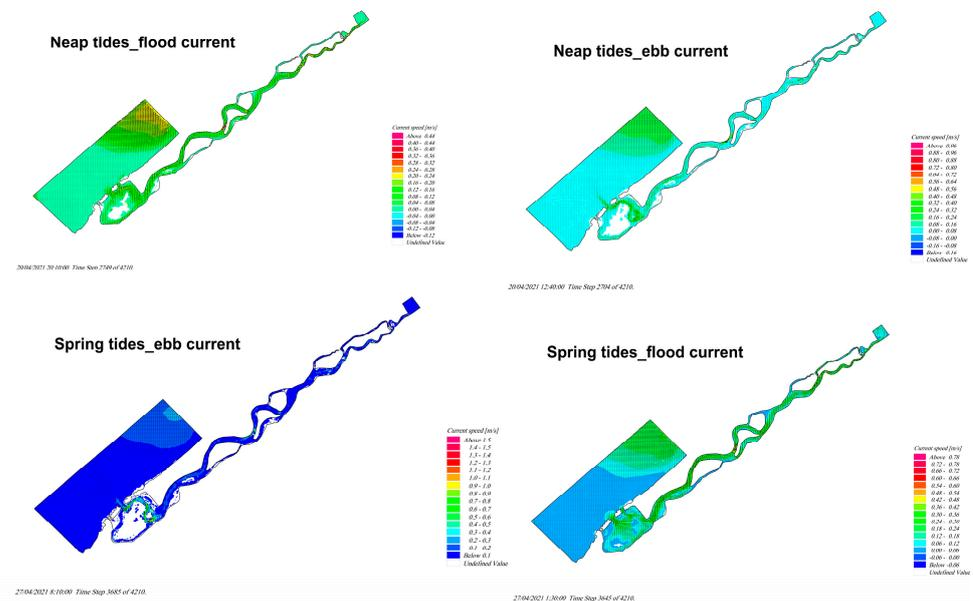
Figure 5. Maps of current velocity simulated during spring and neap tides on April 2021 (Food/ebb).
