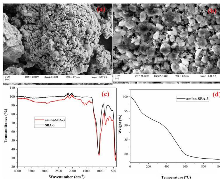
**Figure 1.** Nanosilica morpho-structural characterization: (a,b) SEM images; (c) FTIR spectra; (d) TGA graph.
