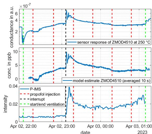
Figure 2. Sensor response of the ZMOD4510 (top), model estimate (middle), and P-IMS (bottom).
