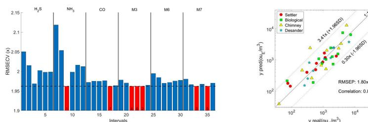
**Figure 1.** (Left) Bar plot displaying the RMSECV at iteration 8 for the addition of a new interval. Red bars are the selected interval. The intervals are 20 s long for each sensor. The first interval for each sensor is synchronized with the activation of the sampler. (Right) Predicted odor concentration vs. real odor concentration (in OuE/m<sup>3</sup>) for the optimal sensor configuration.
