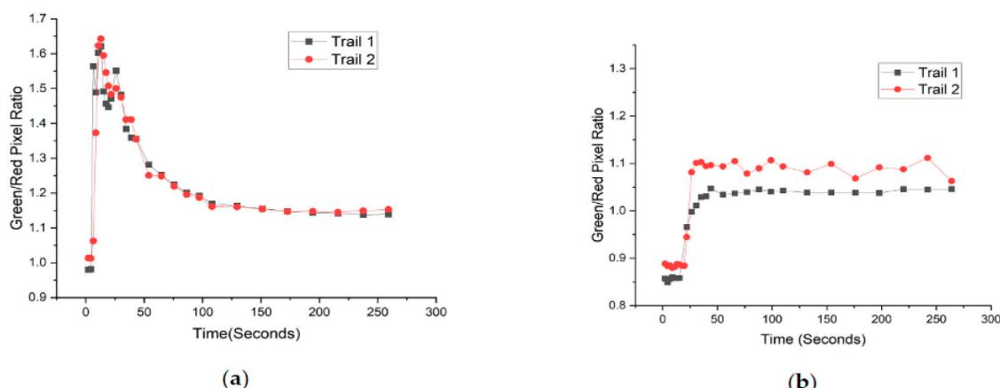
**Figure 2.** Graphs showing time taken to mix: (a) time taken by mp6liq micropump to mix; (b) time taken to mix when a mixing impeller is used.
