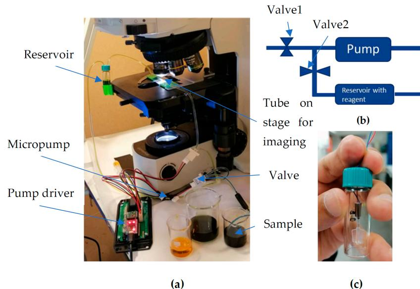
**Figure 1.** (a) Fluidic system under microscope to study mixing; (b) schematic of mixing configuration; (c) impeller designed for mechanical mixing inside the reservoir.
