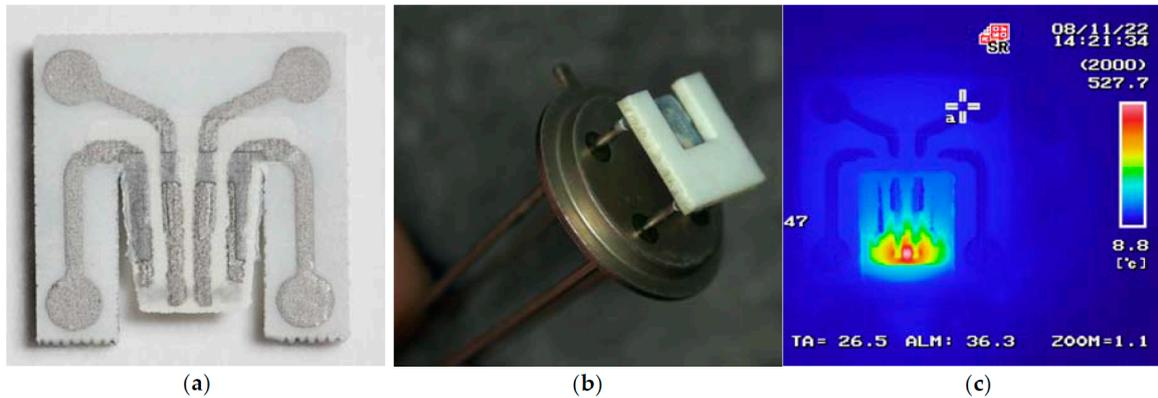
**Figure 1.** Photo of ceramic MEMS sensors fabricated using screen-printing technology. (a) Top view of the microchip with a thin (20  $\mu\text{m}$ ) ceramic cantilever, microheater, and contacts to the sensing layer. (b) Sensor chip packaged into the TO5 housing. (c) Temperature distribution over the microheater and cantilever.
